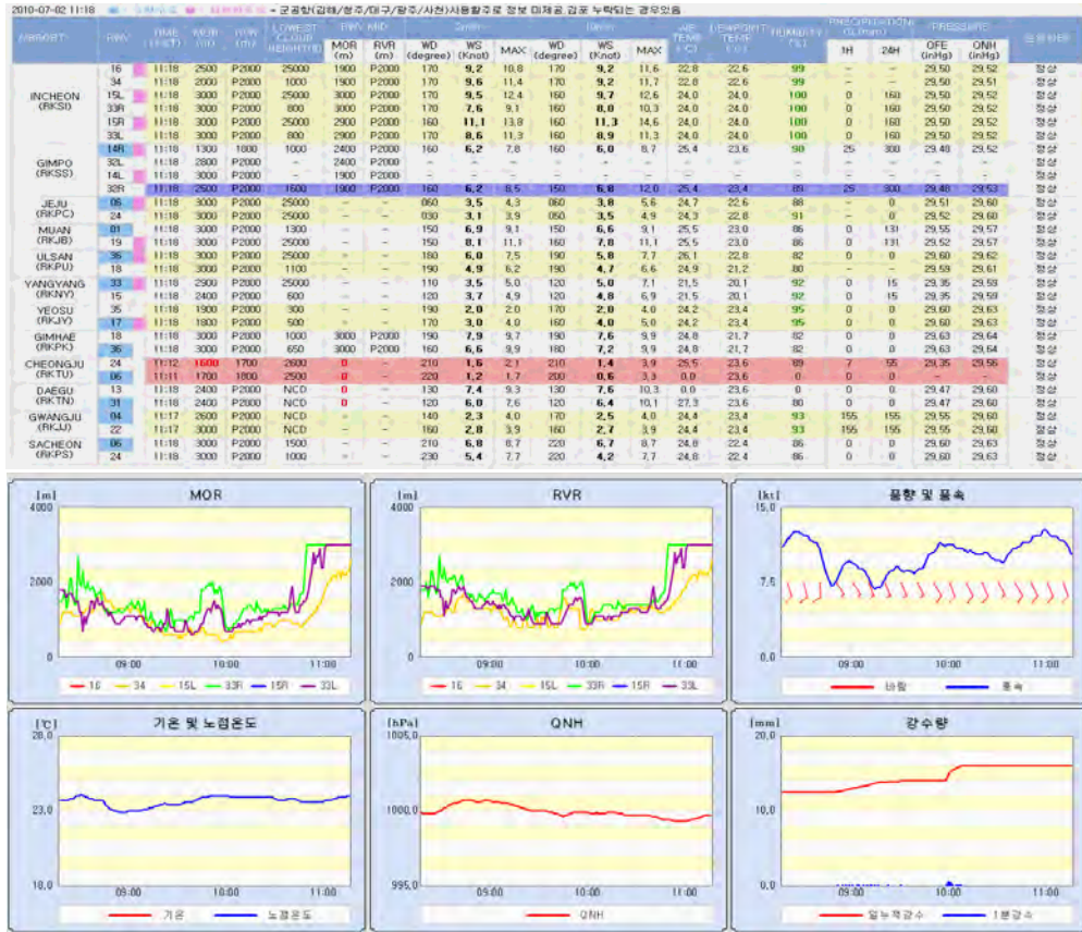
Fig1. Real-time monitoring of AMOS data (alphanumeric and graphic)
