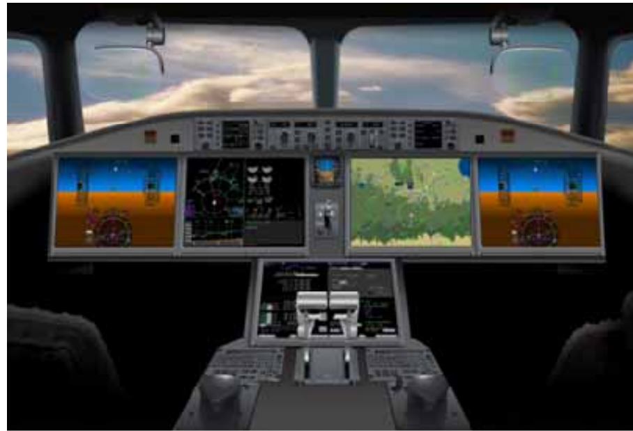
Bombardier C Series Rockwell Collins Pro Line Fusion Flight Deck
