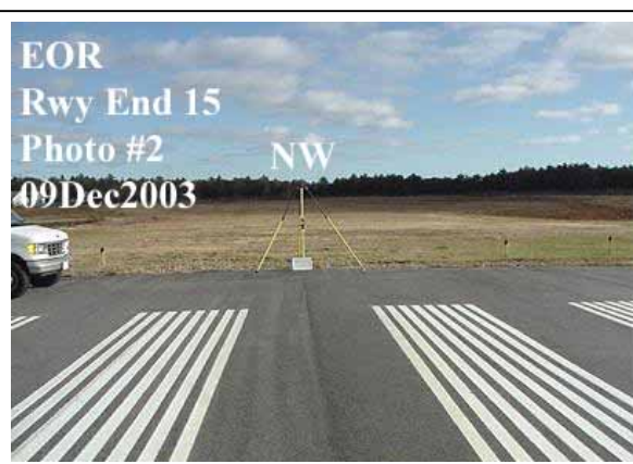
Figure 3-4: Photograph Type #2 (Approach). Photo showing tripod over the mark in foreground and approach in the background.
