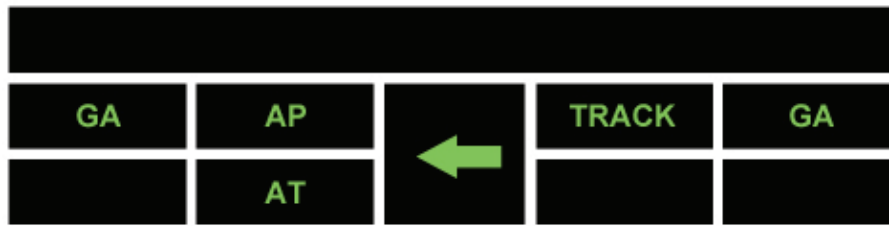
Figure 38 : FMA mode on EMB170
