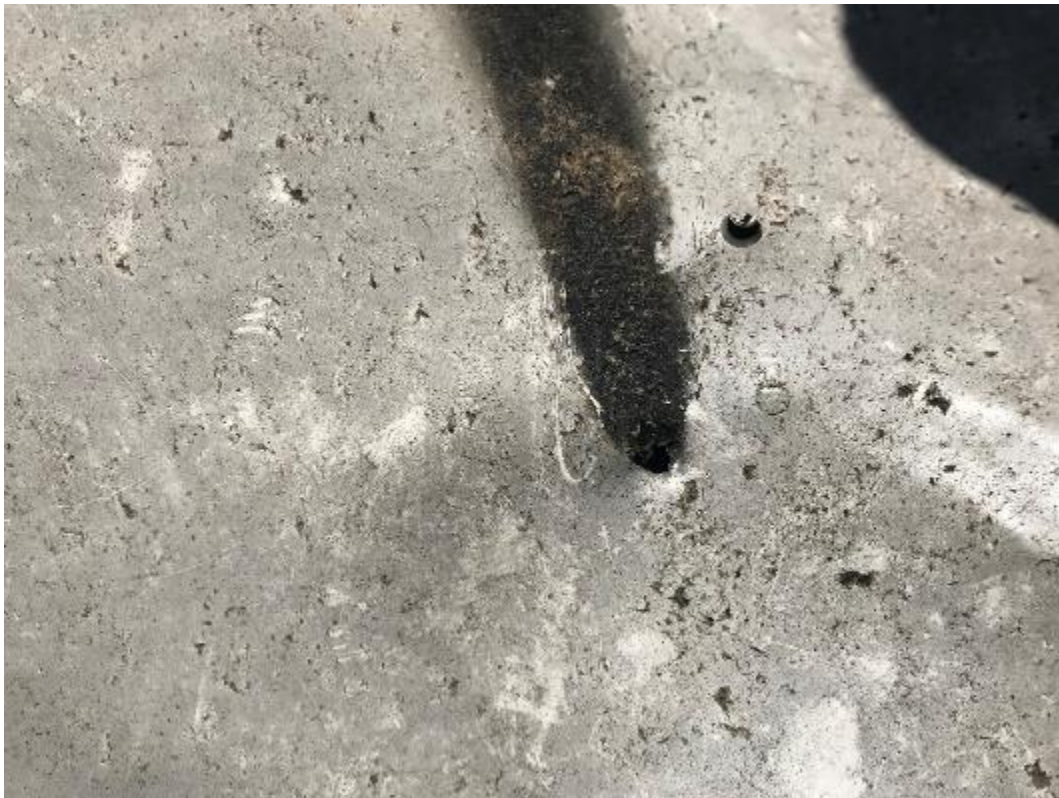
Figure 18- Hole on the fuselage near the cockpit and exhaust fumes
