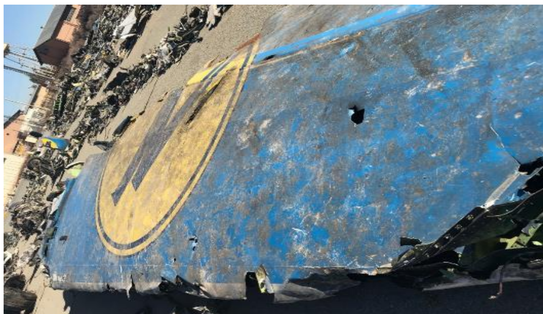
Figure 21- Holes and cracks on vertical stabilizer
