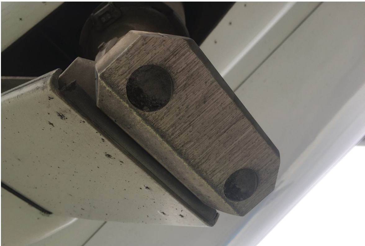
Figure 3: Tail skid shoe with scrape marks.
