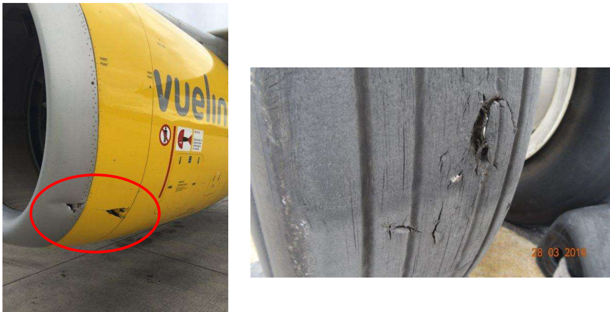
Fig. 10.- Damage to the aircraft
