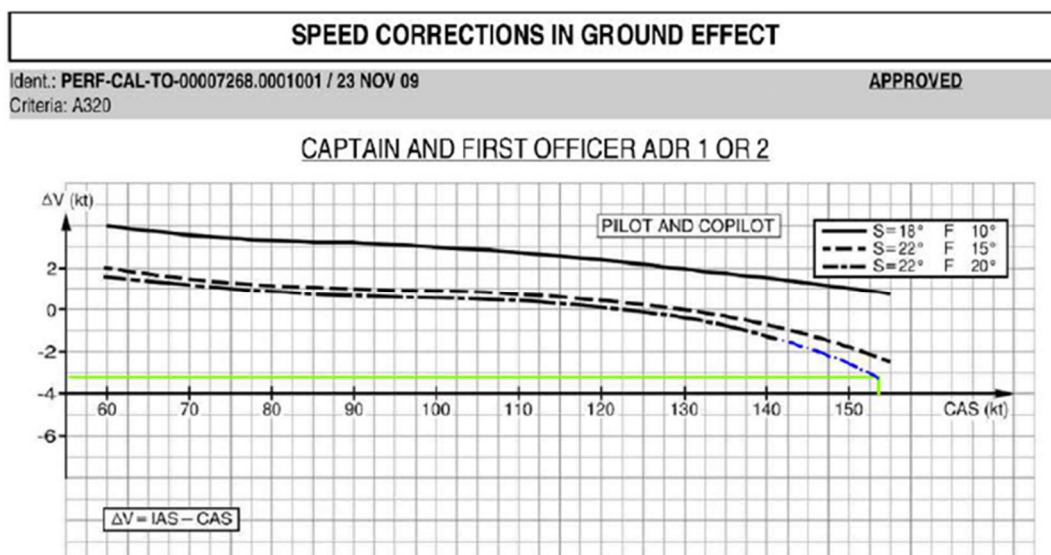
Fig. 8.- Relationship between IAS and CAS in ground effect (Airbus AFM)
