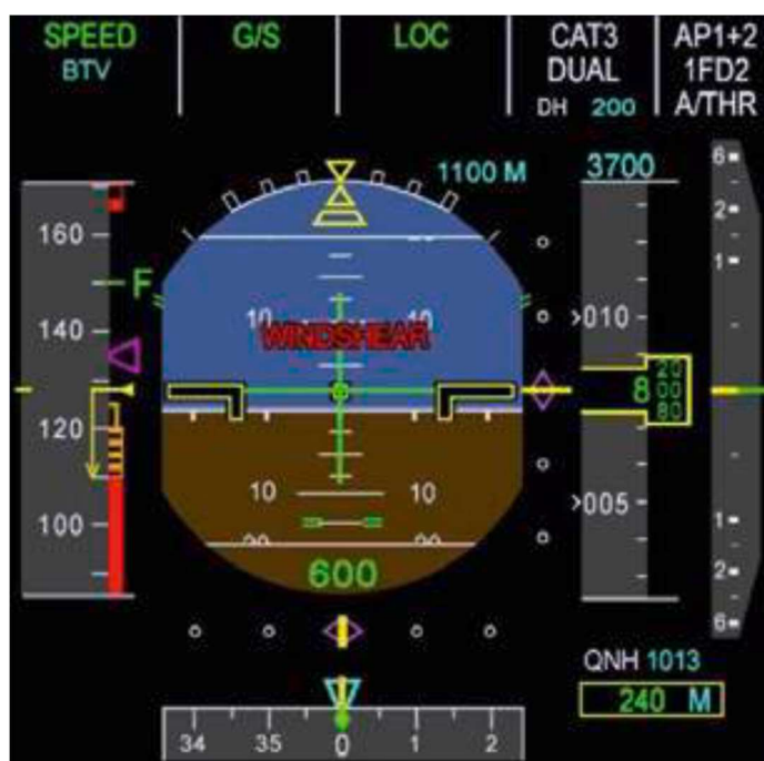
Fig. 3.- Reactive windshear warning indication on the PFD
