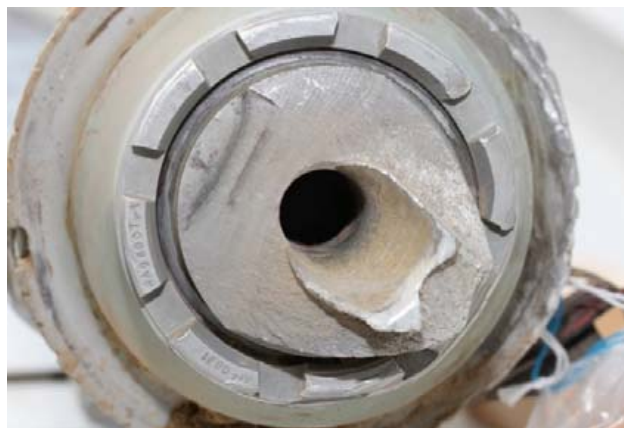
Figure 2: fracture pattern on blade No.2 pre-load bolt
