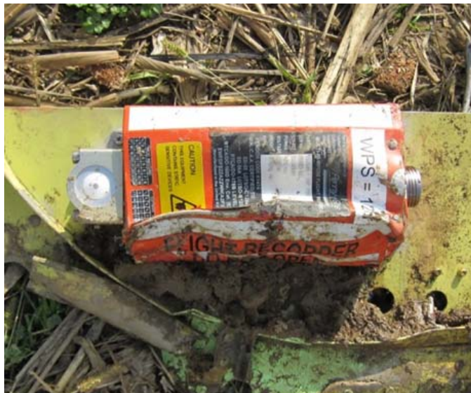
Photo 1: MPFR (combined FDR/CVR) installed on board aircraft AW609 registration marks N609AG.
