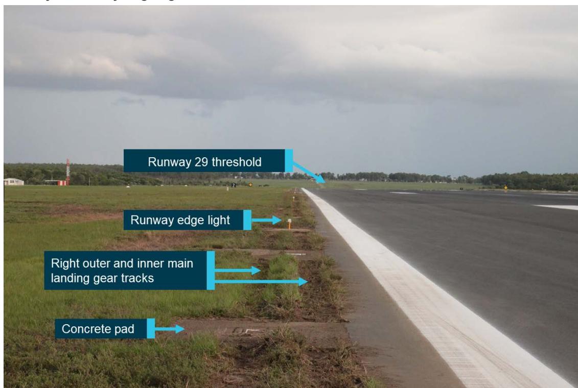
Figure 2: Wheel tracks where VH-VUI departed the runway 29 sealed surface and destroyed runway edge lights 11
