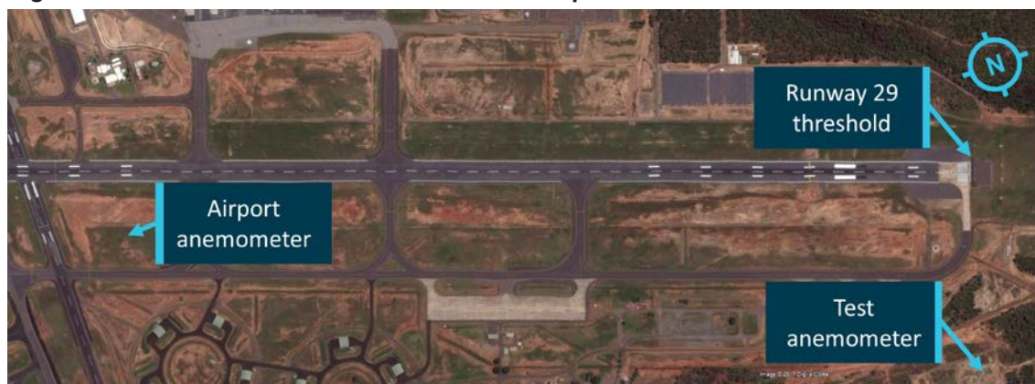
Figure 6: Location of anemometers at Darwin Airport
