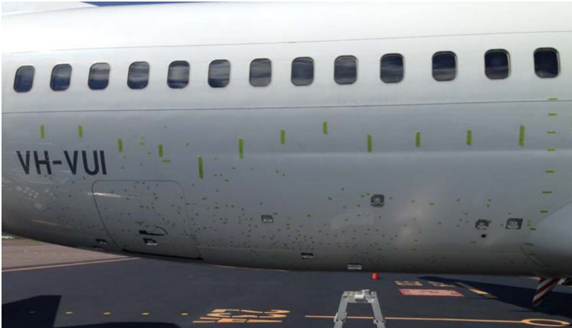
Figure 4: VH-VUI fuselage damage, marked with green tape
