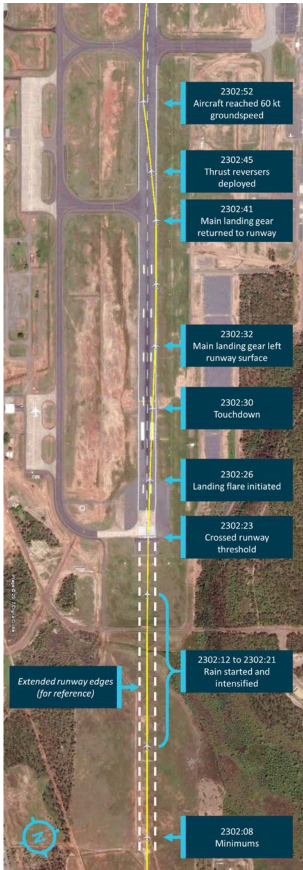
Figure 1: Final approach and landing roll of VH-VUI
