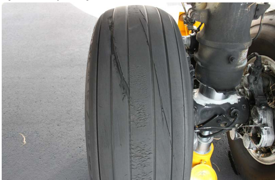
Figure 3: VH-VUI tyre damage
