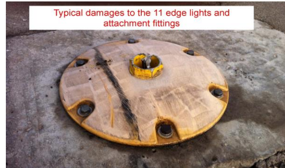
Figure 8. Typical edge light damage
