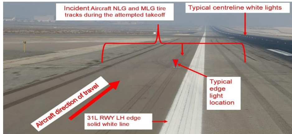
Figure 6. Aircraft NLG and MLG tire tracks
