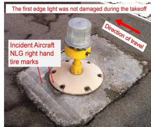
Figure 4. Edge light with tire marks
