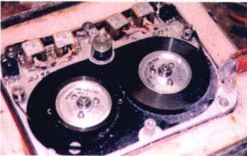
Magnetic tape inside crash protection
