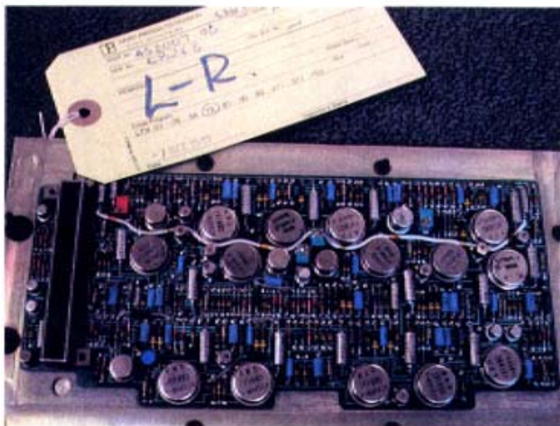
FIGURE 2 Attitude Interface (top) and Attitude Repeater circuit boards
