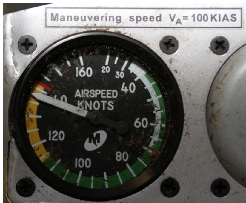
Figure 33: Airspeed indicator markings on instrument
