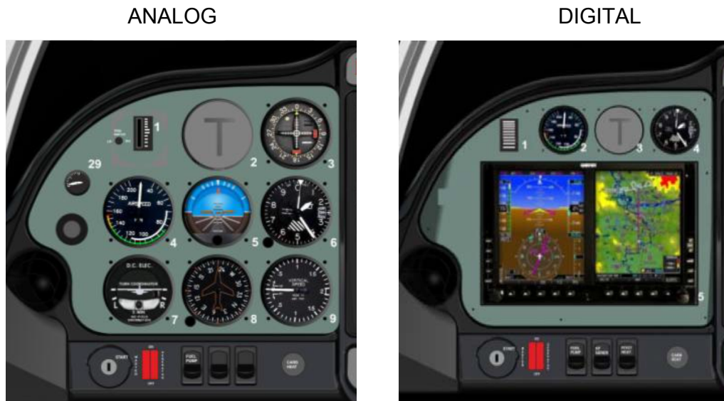
Figure 31: The difference between analog and digital panels
