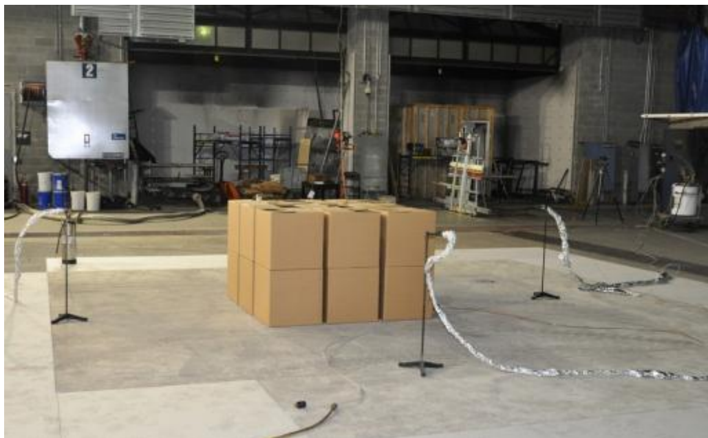
Figure 87: Test setup for tests involving 18 cardboard boxes and one box of batteries
