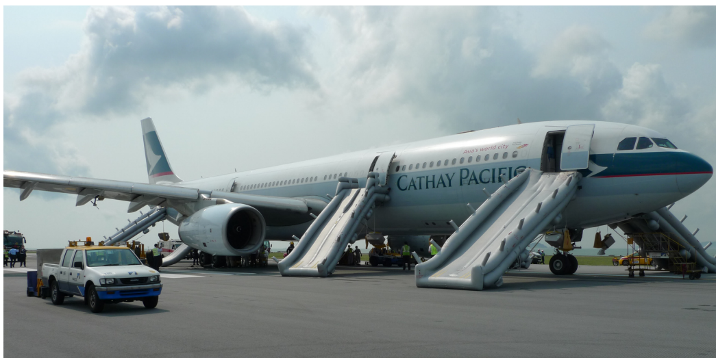
Figure 2: All Emergency Evacuation Slides were deployed
