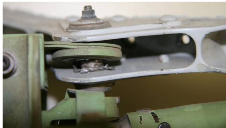
Figure 17: Left Inner Attachment Bearing
