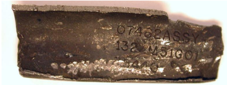
Photo No 4. Piece no 9, HPT Stage 1 Nozzle air cover baffle.
