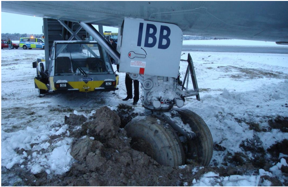
Fig. 51. The nose wheel angled to the right. Photo: Swedavia.
