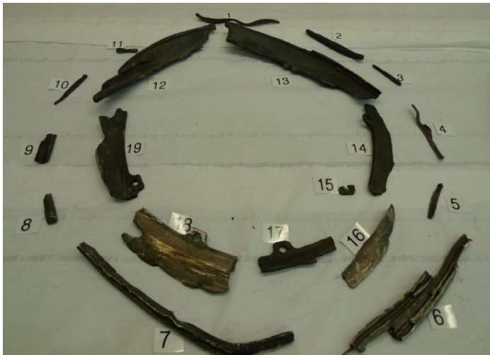
Fig. 42. Fragments of the diffuser aft seal analysed by LHT. Photo: LHT.
