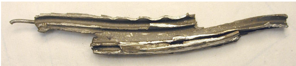
Photo No 5. Piece No 6 is the only fragment with the four seal teeth in the same piece.
