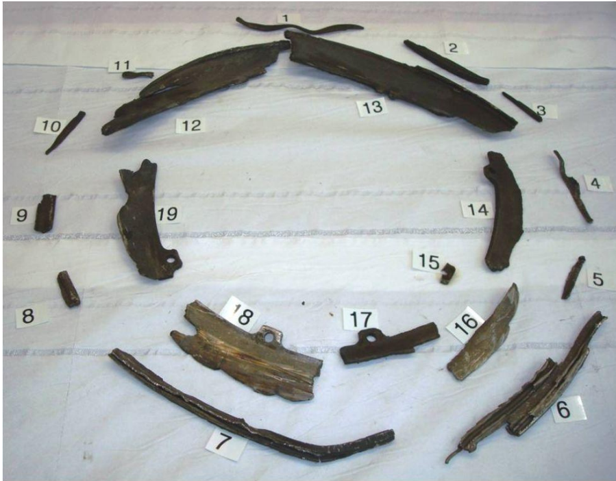
Photo No 2. LHT photo showing Diffuser Aft Seal fragments.
