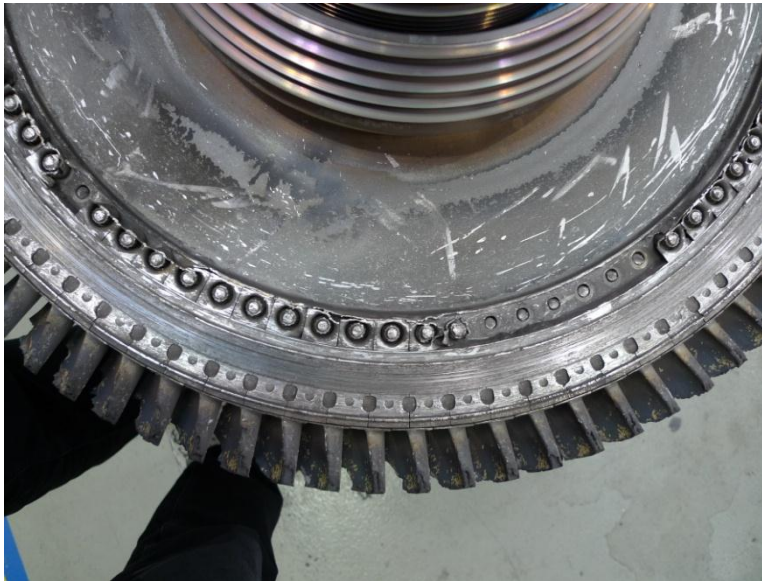
Fig. 38. HPT disc and turbine stage one with Diffuser Front Seal. Photo: SHK.
