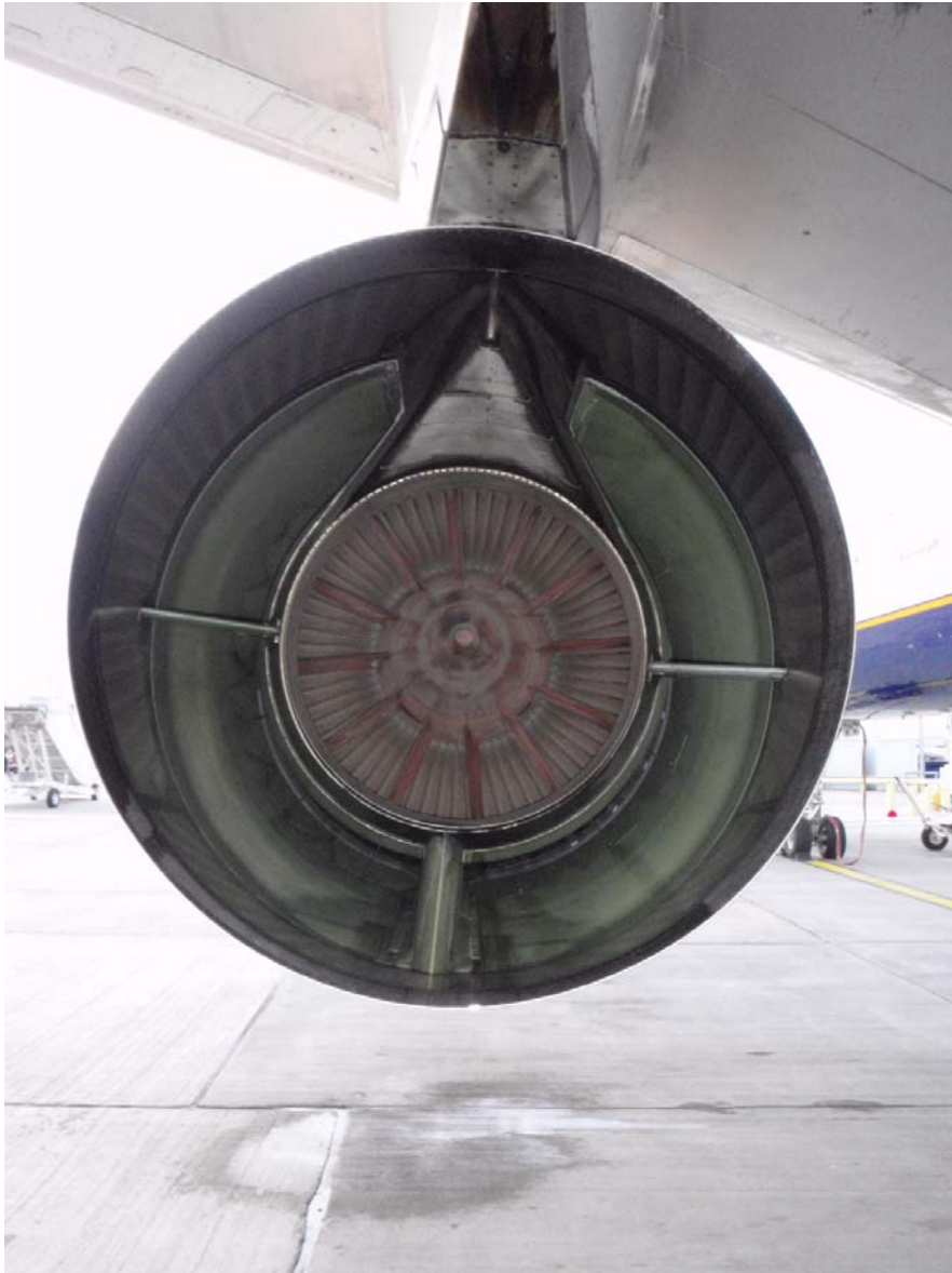
Figure 4 – Fluid seen leaking onto the apron under engine #1
