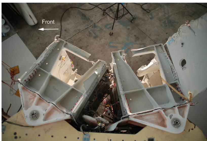
Figure 51: Fin centre and aft attachments
