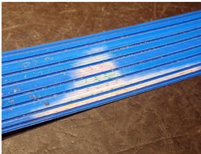
Figure 21: Conductor found exposed on Ribbon 1
