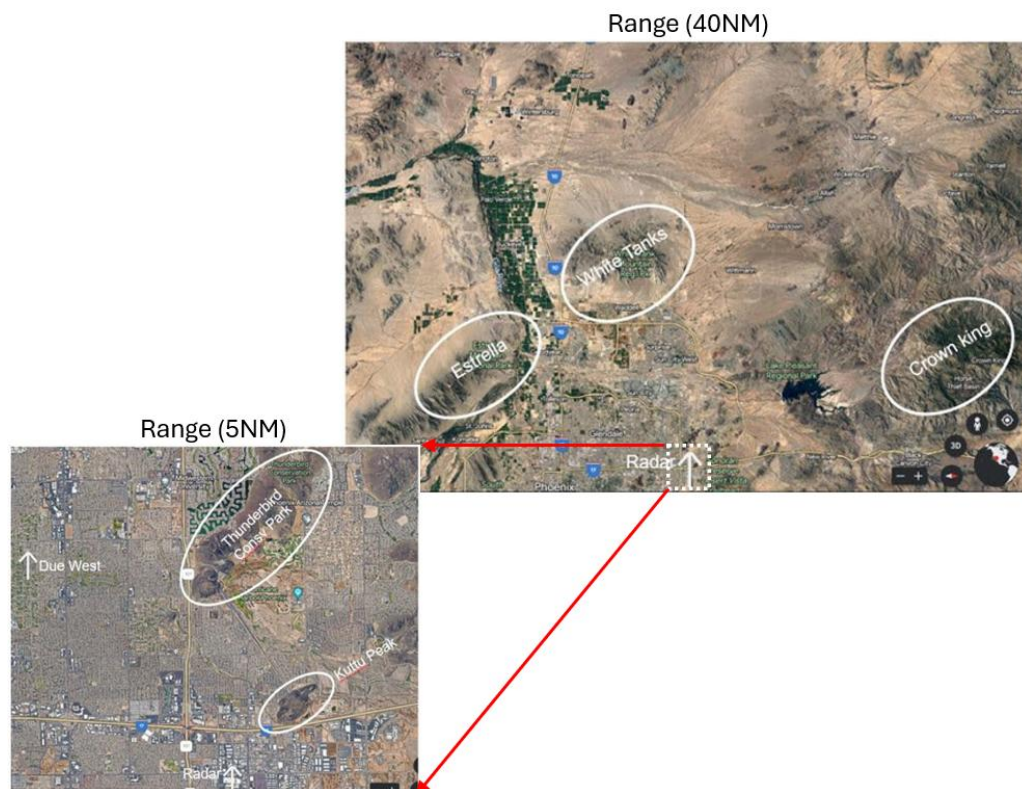
Figure 17: WXR transmission and reception operational test targets
