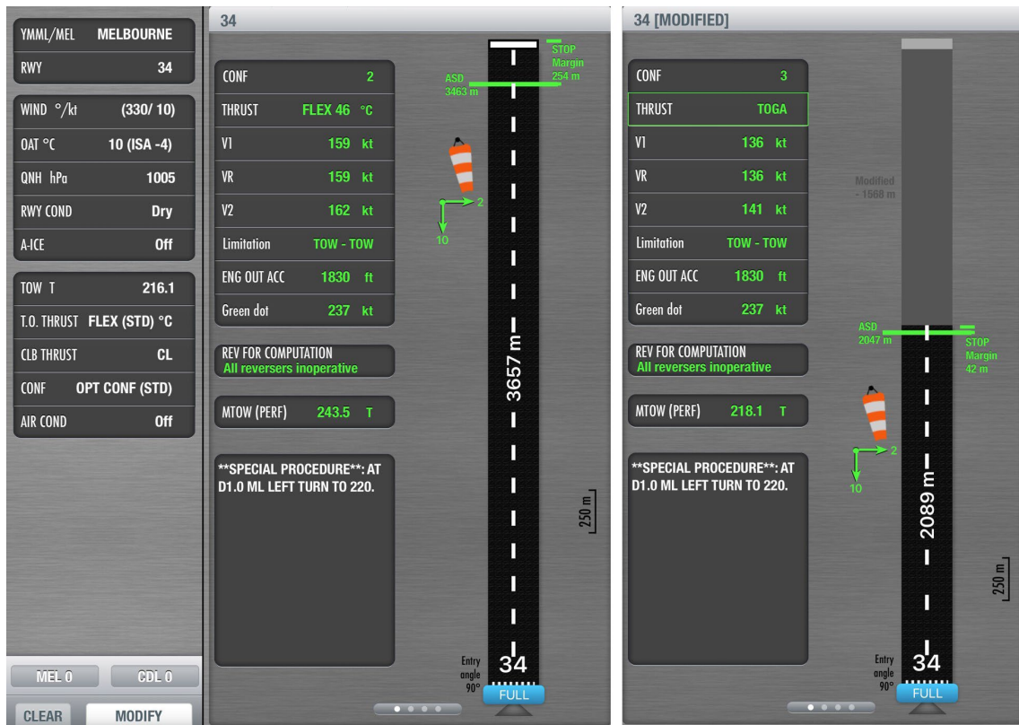
Figure 8: Airbus Flysmart screen images showing performance comparison for 9M-MTL for conditions representative of 7 September 2023. Melbourne runway 34 full-length (centre of image) and reduced-length (right).
