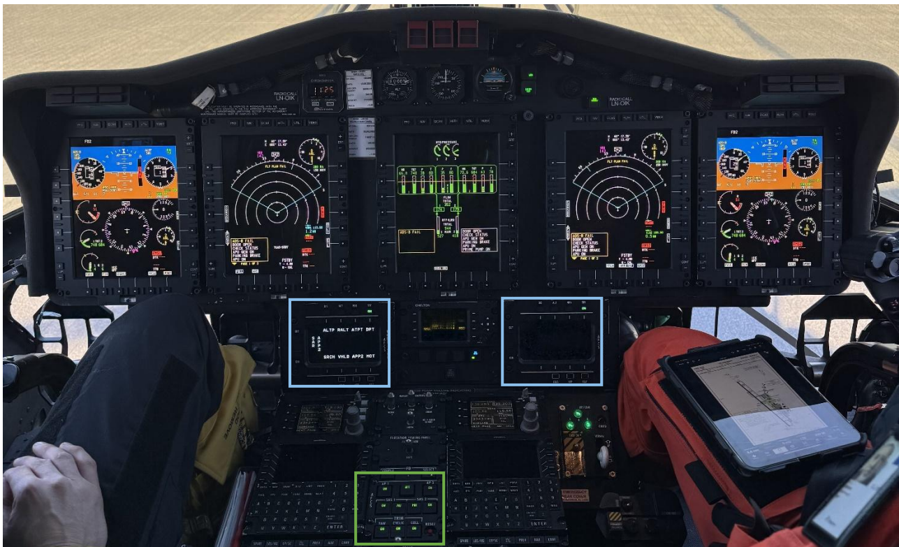
Figure 4: The cockpit of the S-92A. The blue boxes highlight the Mode Select Panels, and the green box highlights the control panel for the Automatic Flight Control System. Photo: NSIA
