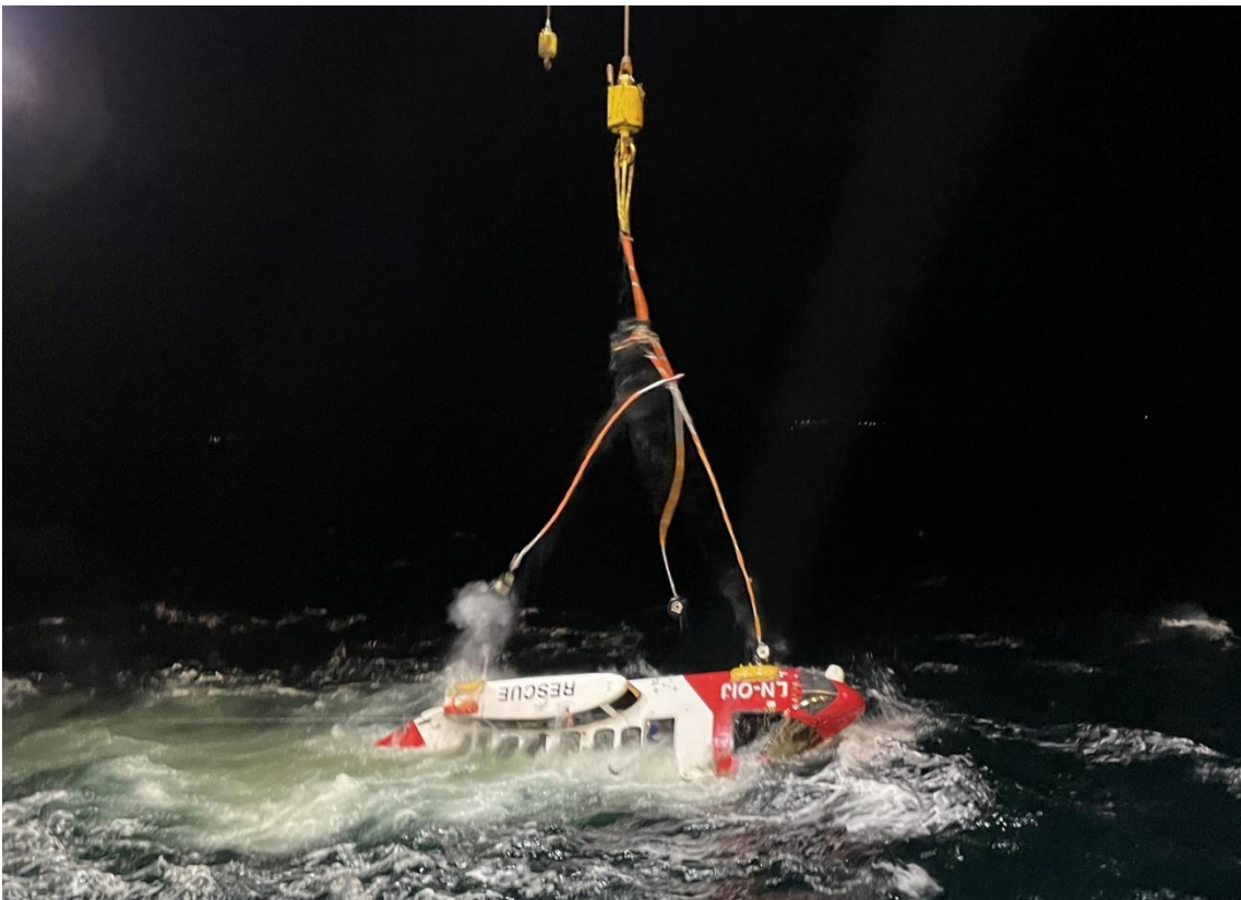
Figure 27: The moment when the left main wheels were pulled loose during first attempt of hoisting the helicopter. Note water flowing through all the windows at the left side. Photo: NSIA
