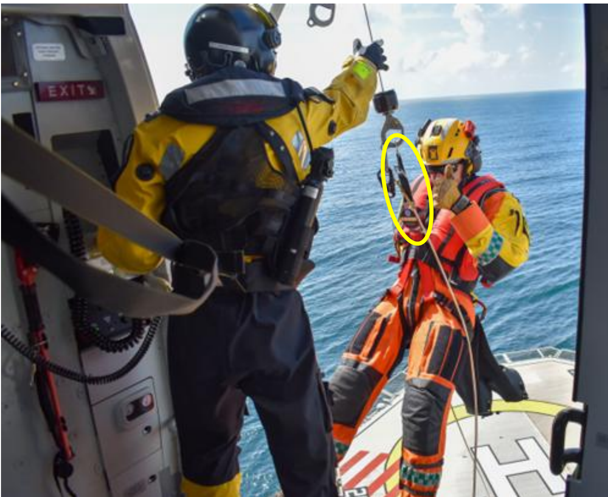
Figure 36: Fully equipped hoist operator secured with a monkey-strap and rescuer with harness hanging in the hoist via a Quick Release Box (inside yellow circle). Photo: Bristow Norway / NSIA
