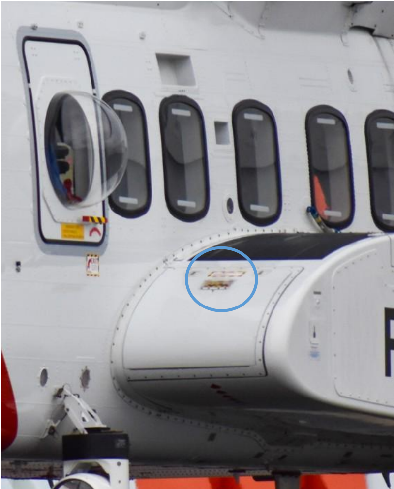
Figure 14: Picture showing the location of the D-ring, blue circle. Photo: Bristow Norway / NSIA
