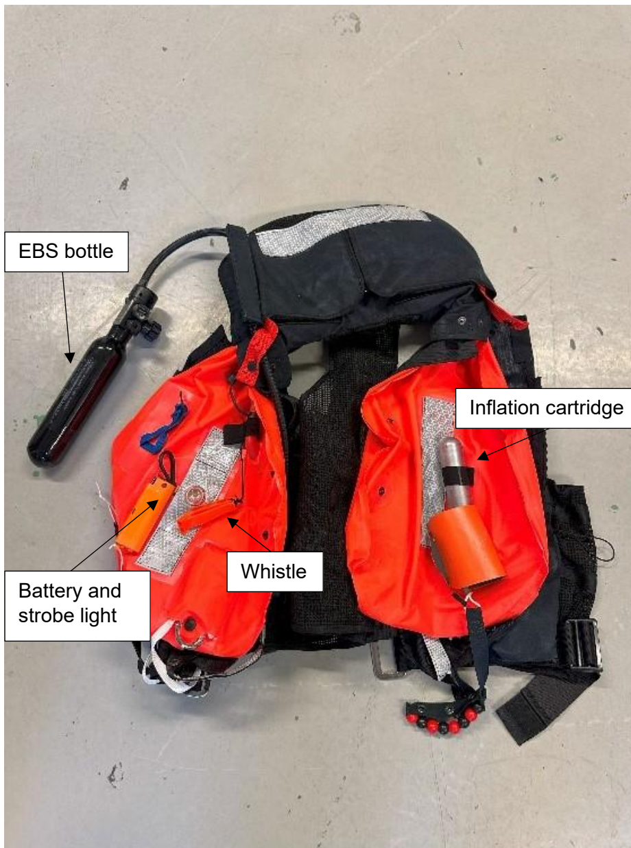
Figure 33: Life jacket type Beaufort MK44 unpacked and with equipment shown. The emergency breathing system bottle to the left in the picture. Photo: NSIA
