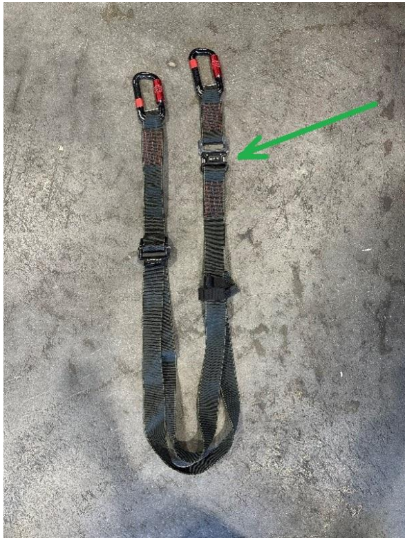
Figure 35: Lanyard with quick-release (green arrow). Photo: NSIA
