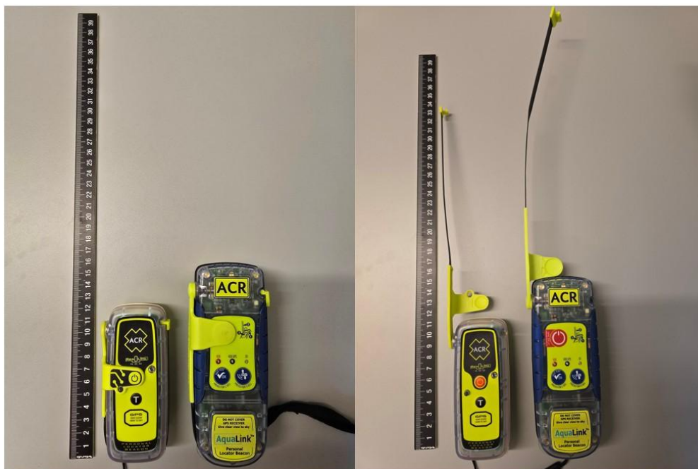
Figure 31: The two types of PLB involved, ResqLink 400 left and Aqualink 350 right in both photos. The photo to the left shows the PLBs with the antenna stowed, and the photo on the right shows the PLBs with the antennas deployed and the red activation button is visible. Photo: NSIA
