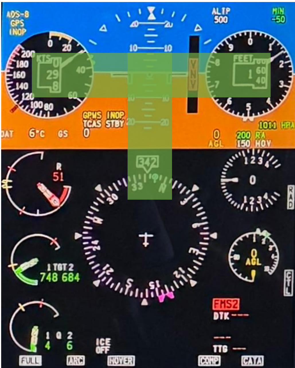
Figure 50: The green T shows the classic T-scan, focused on the attitude indicator, and referencing air speed indicator (left), altitude indicator (right) and heading (down).
