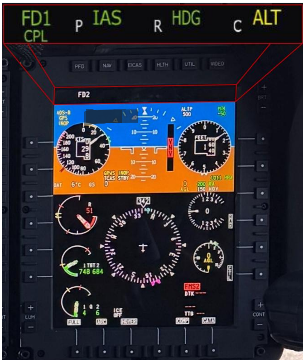
Figure 8: Photo of the Primary Flight Display with an illustration of a degraded collective axis (yellow ALT). A strip on the PFD with flight director annunciators is expanded and highlighted with red lines. Photo: NSIA. Illustration: Sikorsky/NSIA
