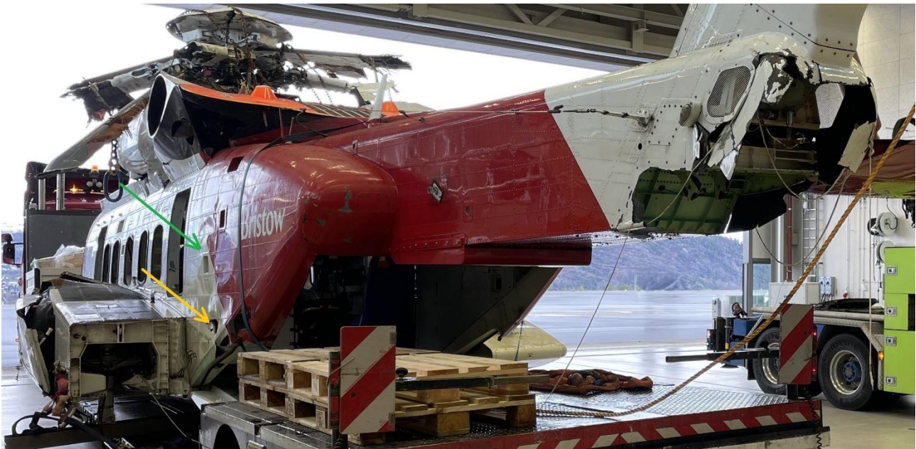
Figure 29: The helicopter seen from the aft left quarter. The aft part of the left sponson is missing. A hole on the fuselage side adjacent to the sponson indicate that the missing part was forced into the fuselage (yellow arrow). The green arrow points towards hydro deformation. Also noticeable is the missing aft door and the damaged tail boom. Photo: The NSIA
