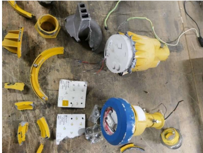
Figure 11: debris from the destroyed lights
