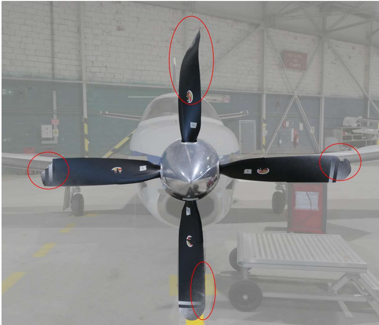
Figure 3: view of the damaged propeller
