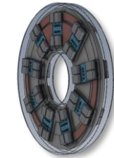
High Voltage / Cryocooled Power Electronics > 50 KW/KG
