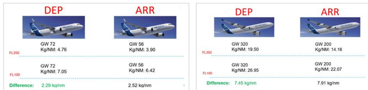
Figure 15: inverse Specific Range differential between cruise (FL 350) and FL100 for departure (DEP) and arrival (ARR) for two different aircraft types: a typical single-aisle aircraft type (left side) and typical wide-body aircraft (right side)
