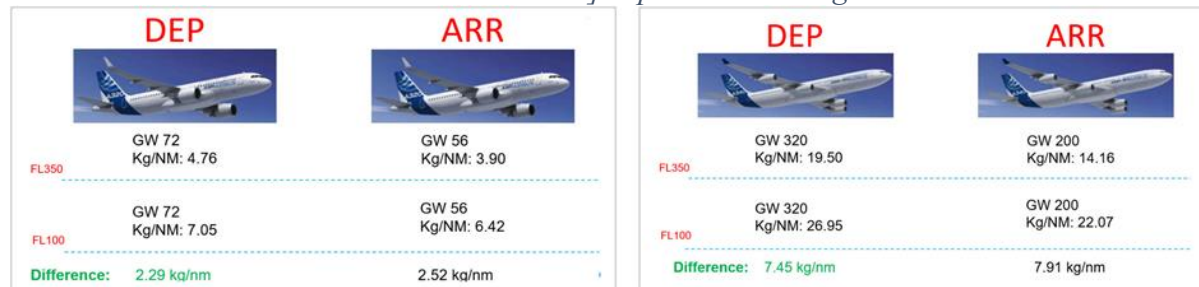
Figure 15 between optimum and sub-optimum flight levels for two aircraft representatives of single-aisle and wide-body aircraft. The fuel burn differential is showed as the inverse specific range differential, which is the amount of fuel burn per unit of flown distance.
