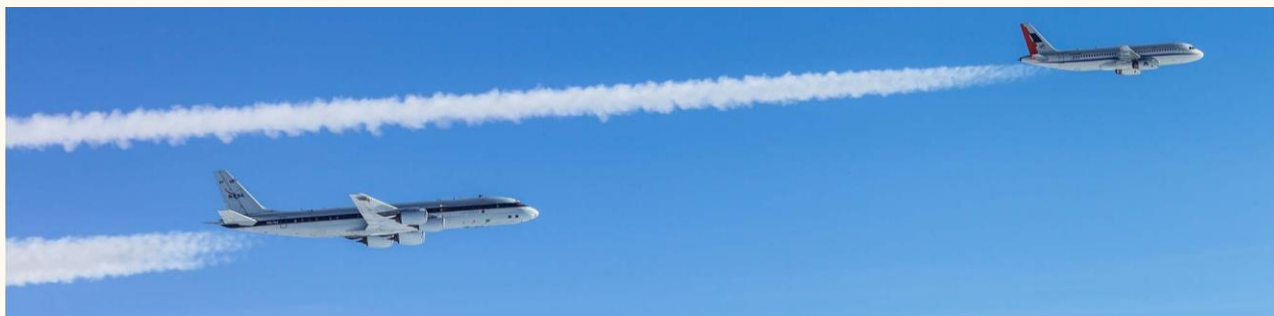
DC8 chasing a contrail from the A320 burning a SAF blend above Germany, 24 January 2018
