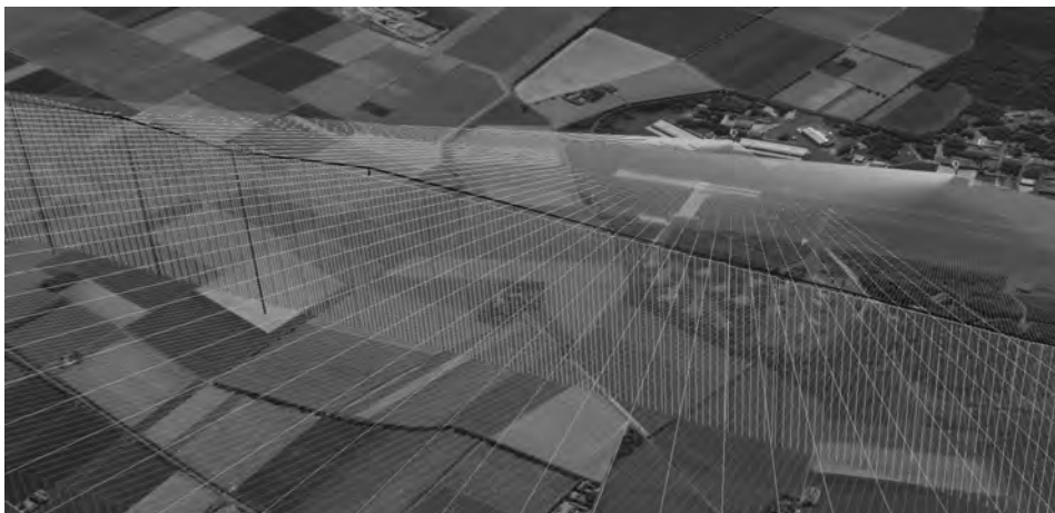
Figure 6. Reconstructed flight path (black line), lines of sight (grey lines), and radar data (grey path).
