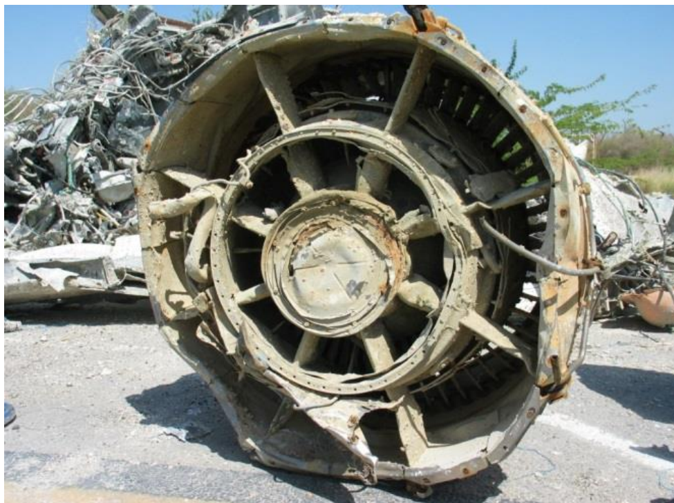
Impact evidence on the lower right hand side of the right engine
