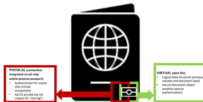
Figure 1 – eMRTD – Physical and Virtual Components
