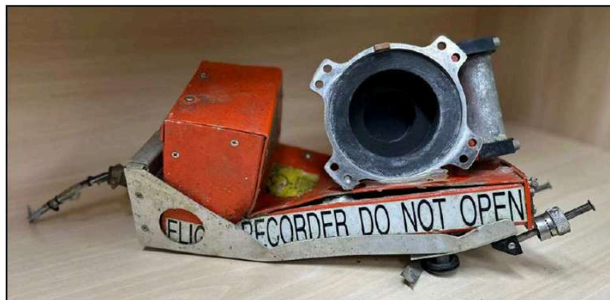
Figure 30 - Cockpit Voice Recorder installed in the PS-VPB.
