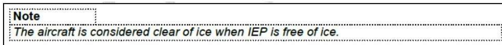
Figure 5 - Note extracted from the procedure related to Icing Conditions of the ATR 72-212A AFM.
