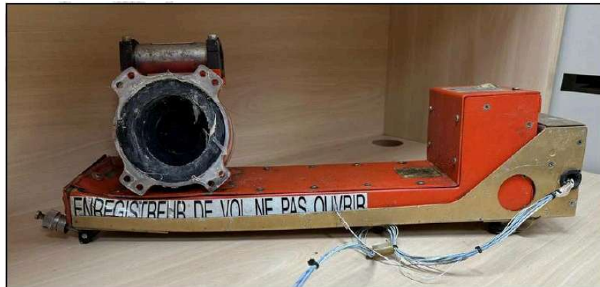
Figure 29 - Flight Data Recorder installed in the PS-VPB.
