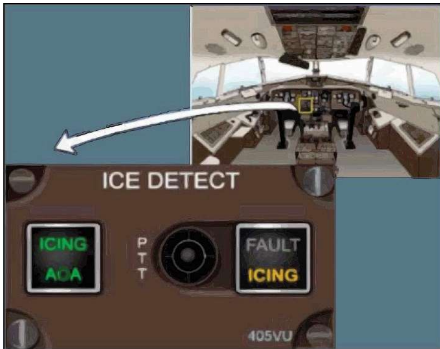
Figure 8 - Indication of the ICE DETECT panel with the amber light illuminated, showing an "ICING" condition.
