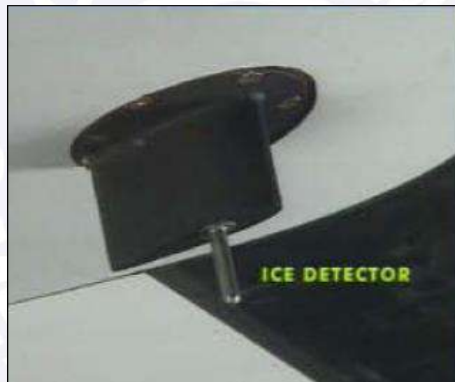
Figure 17 – Electronic Ice Detector. Source: Systems_42-500_72-500 ATR Training & Flight Operations Services.
