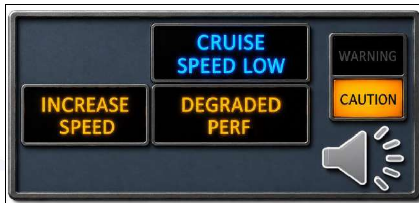
Figure 186– APM INCREASE SPEED alert, associated with MASTER CAUTION alert, accompanied by a single chime aural alert.
