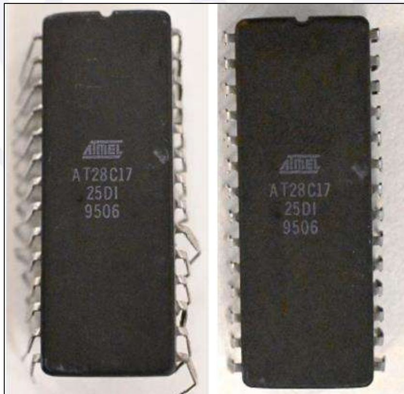
Figure 59 – On the left, MFC1B memory with damaged pins; on the right, the same component after pin repair for the execution of tests and data readout.
