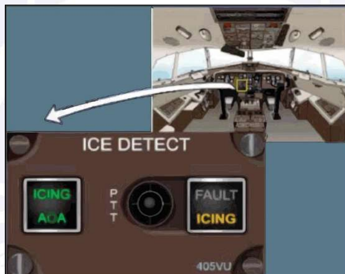
Figure 22 – Indications of the ICE DETECT panel. Source: ATR Training Centre.
