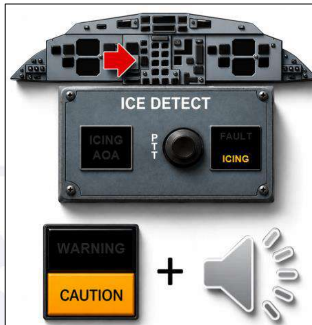
Figure 181 - MASTER CAUTION alert, accompanied by the single chime aural warning, associated with the illumination of the ICING light.
