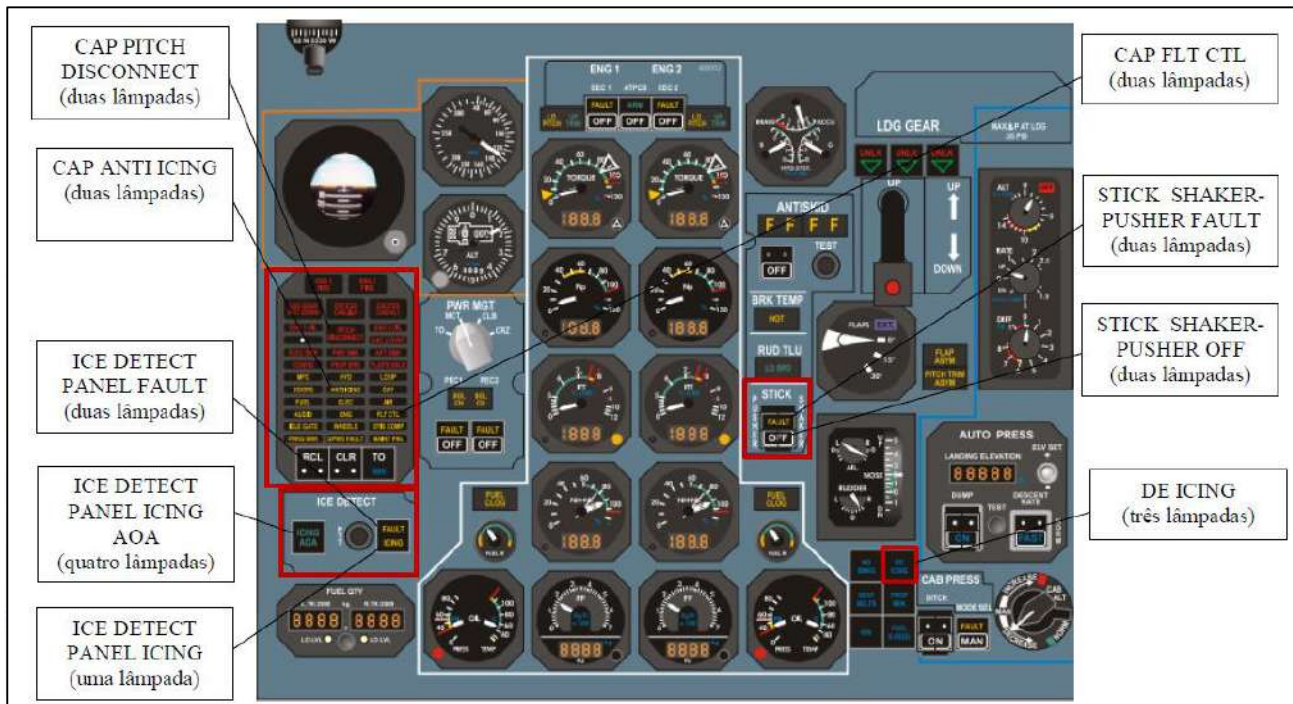
Figure 75 – Central panel showing the positions of the indicator lights from which the lamps were removed for laboratory examination.
