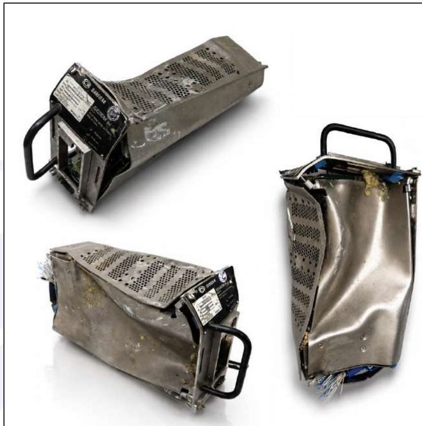
Figure 65 – Images of the MPC installed on aircraft PS-VPB, showing damage and deformation of its housing.
