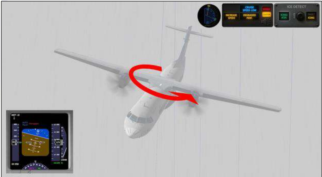
Figure 194 - Illustration demonstrating the aircraft in a flat spin.
