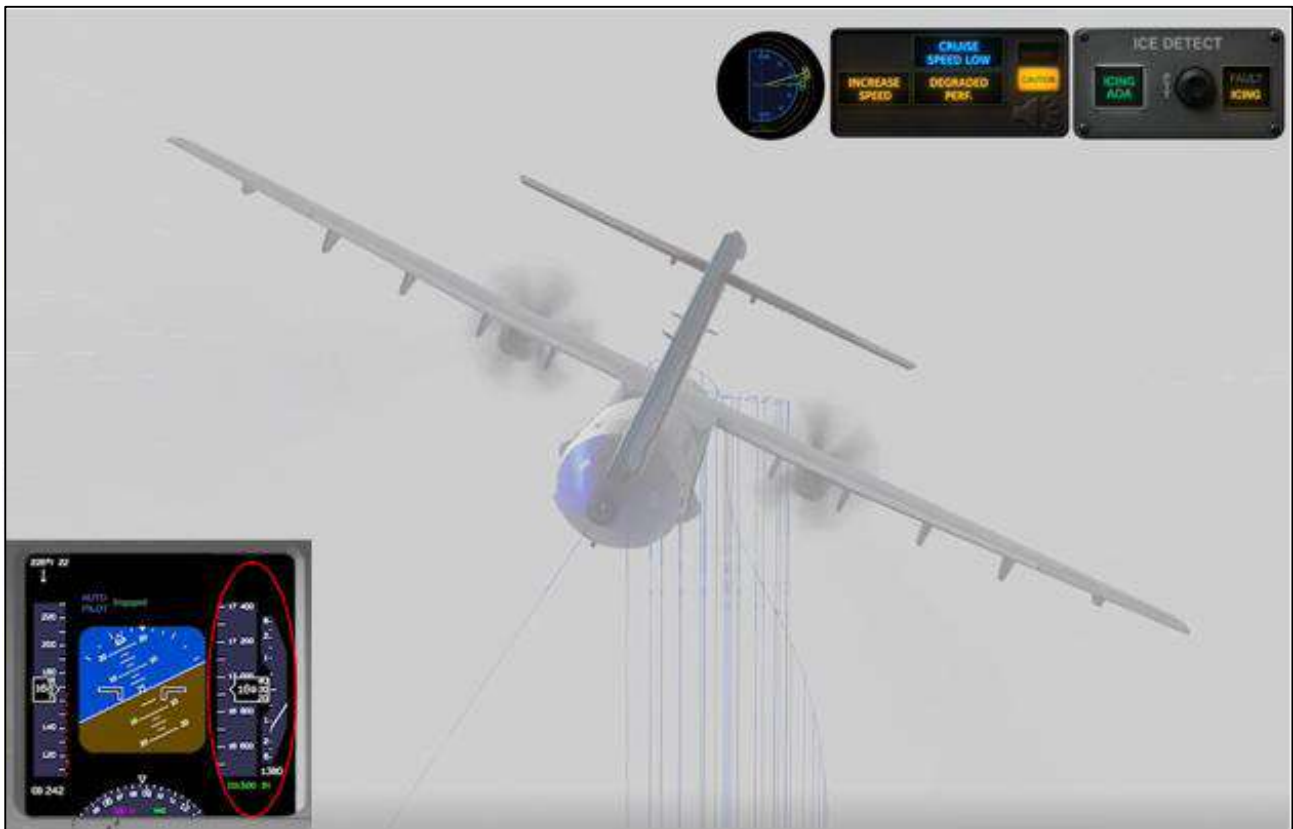
Figure 187 - Illustration demonstrating the altitude loss during the turn due to performance degradation, with the AP engaged in ALT HOLD and the lateral bank in HIGH BANK mode.
