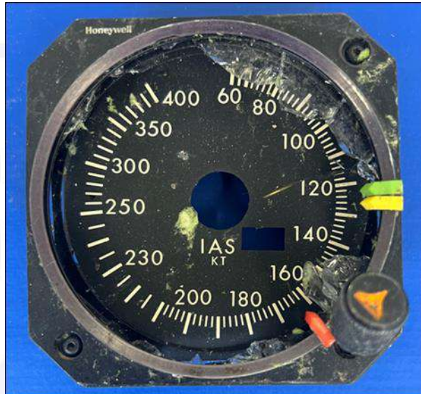
Figure 161 – PIC's airspeed indicator with the RED BUG set to a speed close to 165 kt.
