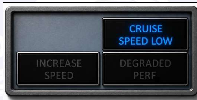
Figure 183 - CRUISE SPEED LOW alert on the left-side APM panel (PIC).
