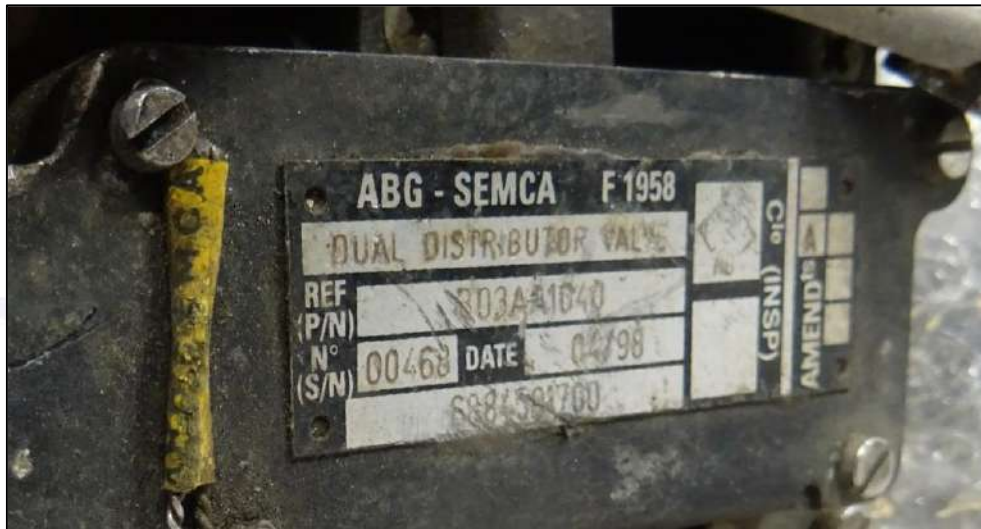
Figure 104 – DDV, FIN 11DM, Identification Plate.
