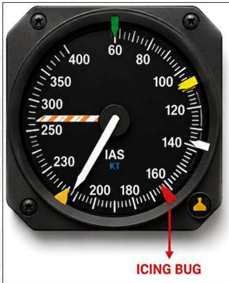
Figure 25 – Airspeed Indicator of the ATR-72-212A, highlighting the ICING BUG.
