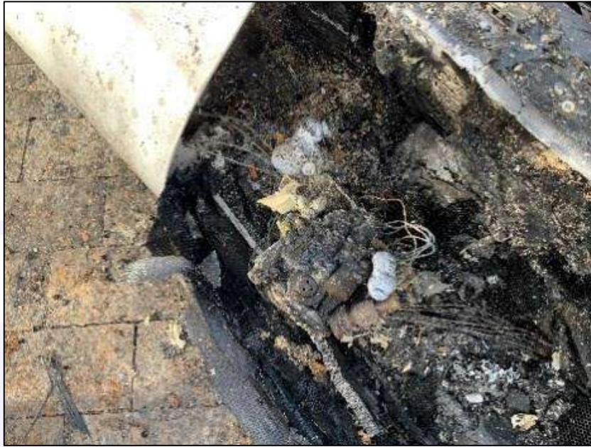
Figure 107 – Image of the FIN 10DM DDV at the crash site.
