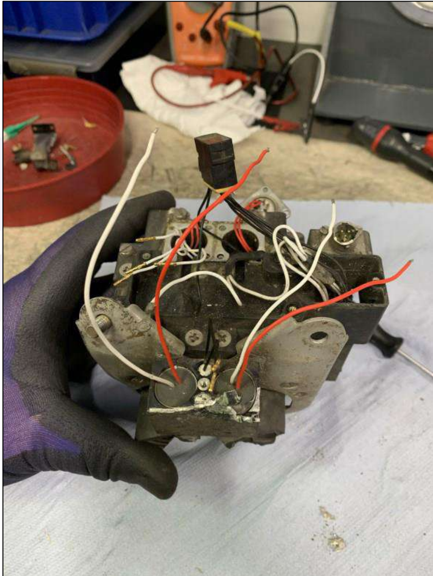
Figure 106 – DDV responsible for actuating the horizontal stabilizer boots subjected to examination.
