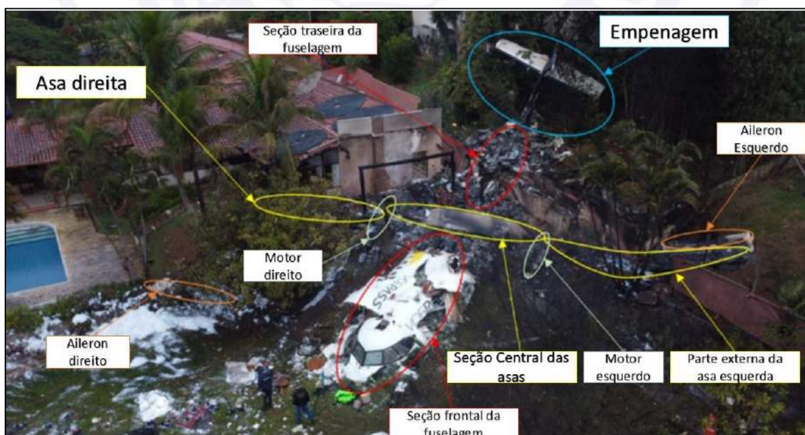
Figure 52 – Illustration showing the location of aircraft components after the impact.
