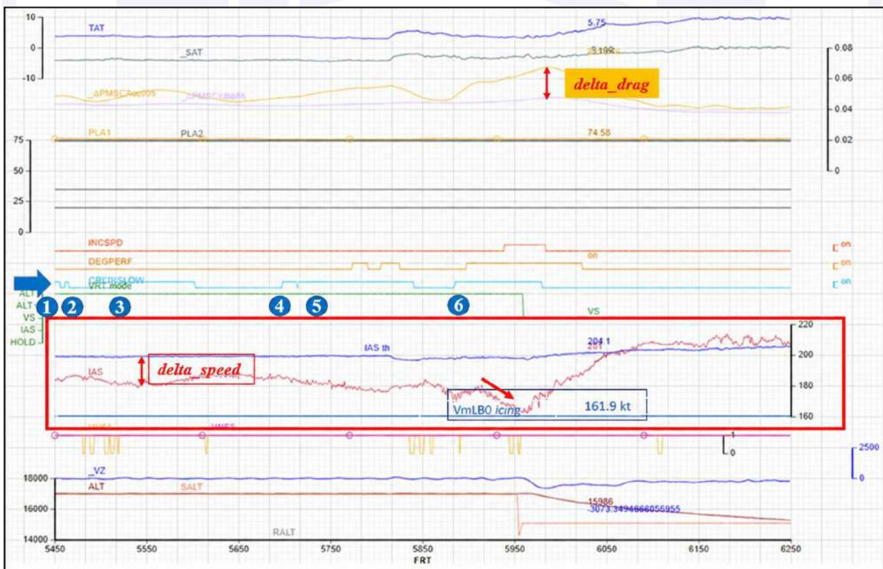
Figure 196 – Graphs reproduced from Figure 130 of this Report. Indication of Delta_Speed around 20 kt throughout the entire cruise phase, with 6 activations of the CRUISE SPEED LOW advisory.
