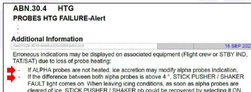
Figure 100 –Arrows indicating additional information contained in the ABN 30.4 of the aircraft FCOM.
