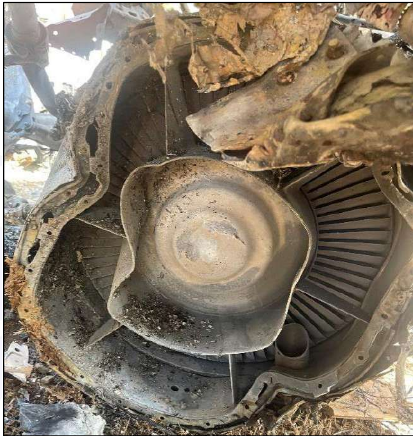
Figure 115 – Rear view of engine No. 1, showing deformations in the turbine support casing and the blades of the 2 nd stage of the power turbine.
