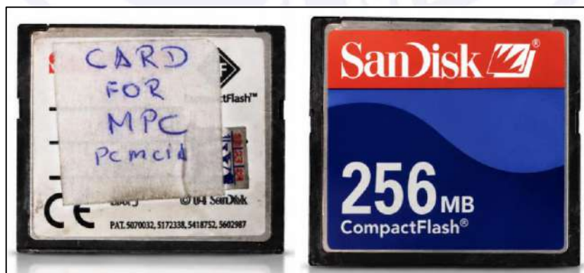
Figure 67 - On the left, rear face; on the right, front face of the PCMCIA card removed from the MPC slot of aircraft PS-VPB.
