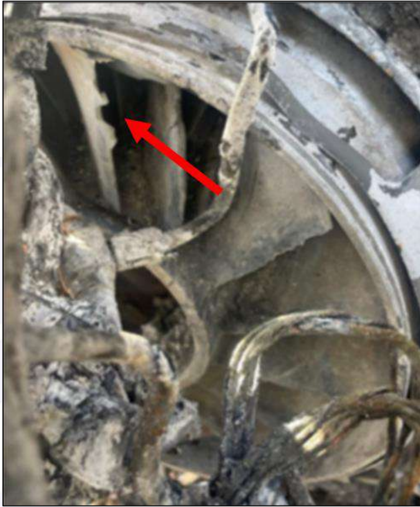
Figure 111 – Image of the LPC rotor of engine No. 1. Red arrow indicating blade deformations in the direction opposite to the rotation of the rotor shaft.
