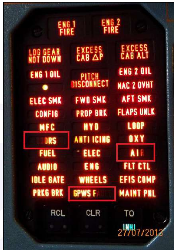
Figure 88 – Example image of a CAP in test mode, showing three indications in which only one of the lamps was illuminated.
