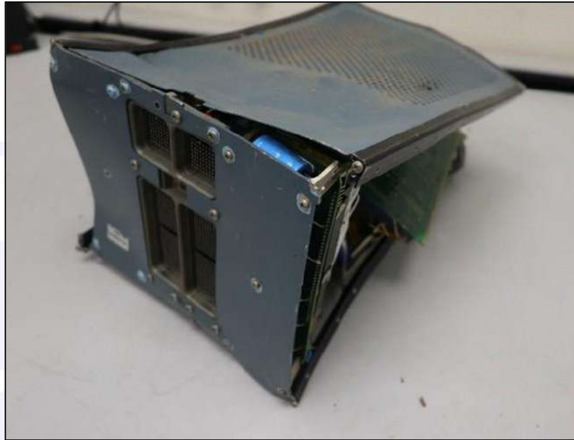
Figure 60 – General condition of the MFC2 prior to disassembly.
