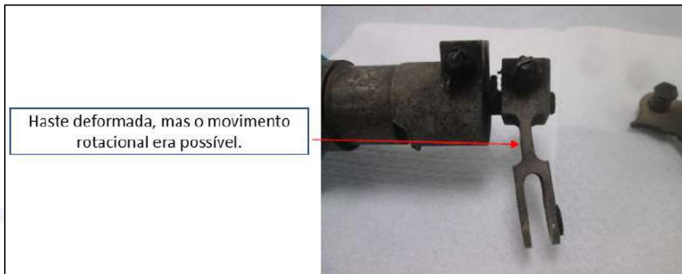
Figure 96 – Synchro transmitter linkage rod deformed, yet still functional.
