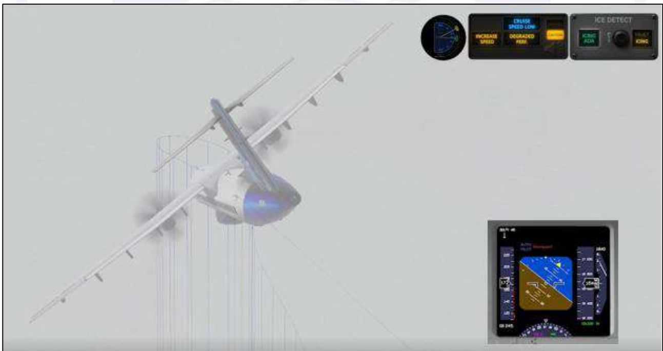
Figure 190 - Illustration demonstrating the stick pusher activation during the reversal turn to the right.
