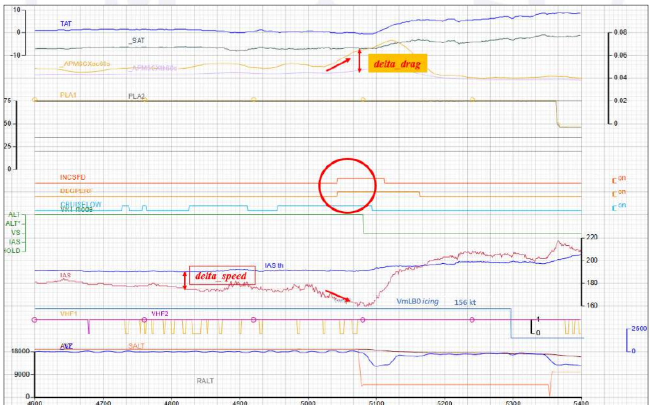
Figure 198 - Flight data graphs reproduced from Figure 131 of this Report, showing delta_speed during the cruise phase and the simultaneous activation of the DEGRADED PERFORMANCE and INCREASE SPEED alerts following the increase in delta_drag.
