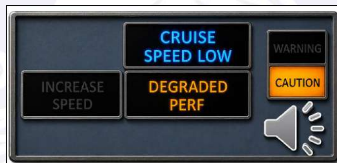
Figure 184 - DEGRADED PERFORMANCE APM alert associated with MASTER CAUTION, accompanied by the single chime aural warning.
