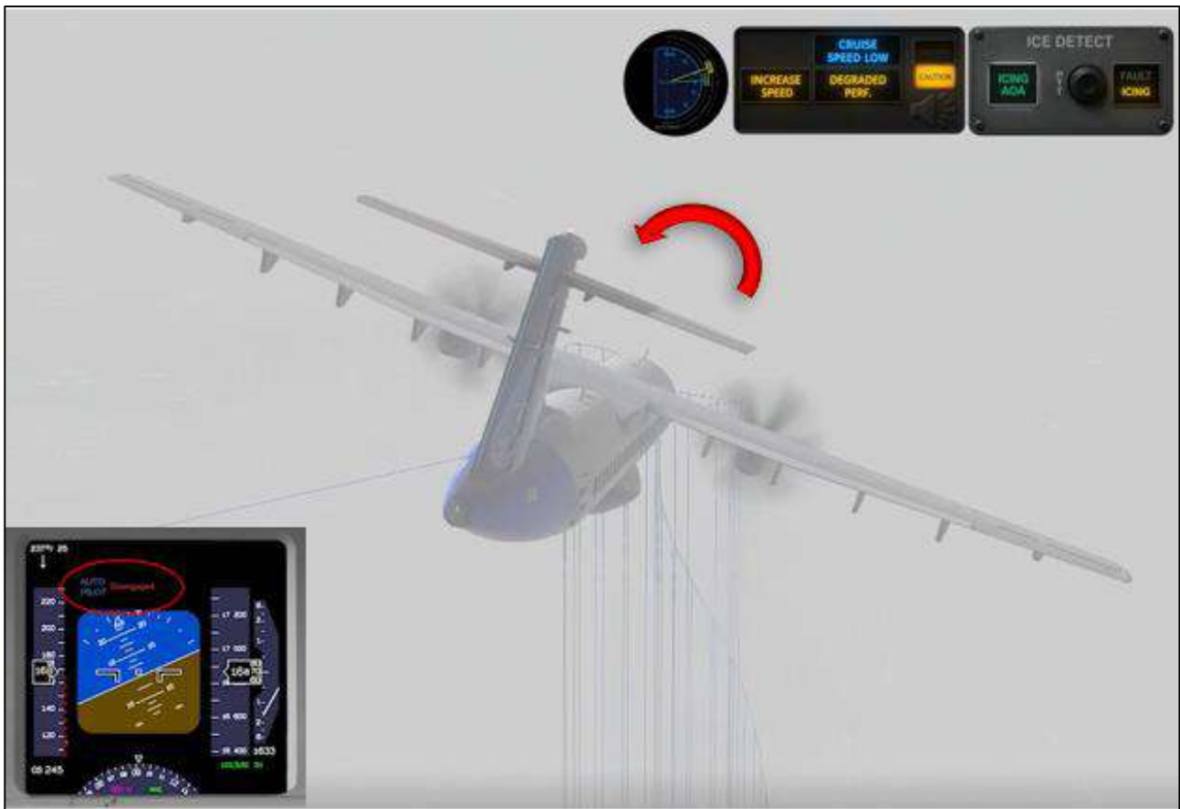
Figure 188 - Illustration demonstrating the moment of stick shaker activation and AP disengagement.
