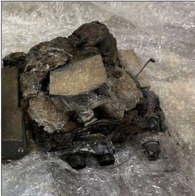
Figure 108 – Photograph of the DDV responsible for actuating the outer boots of the right wing on the test bench for analysis.
