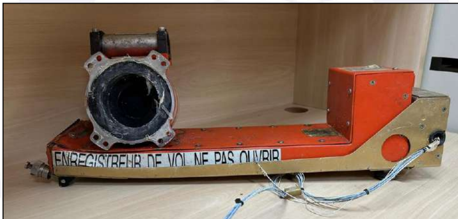
Figure 47 – FDR of the PS-VPB aircraft.
