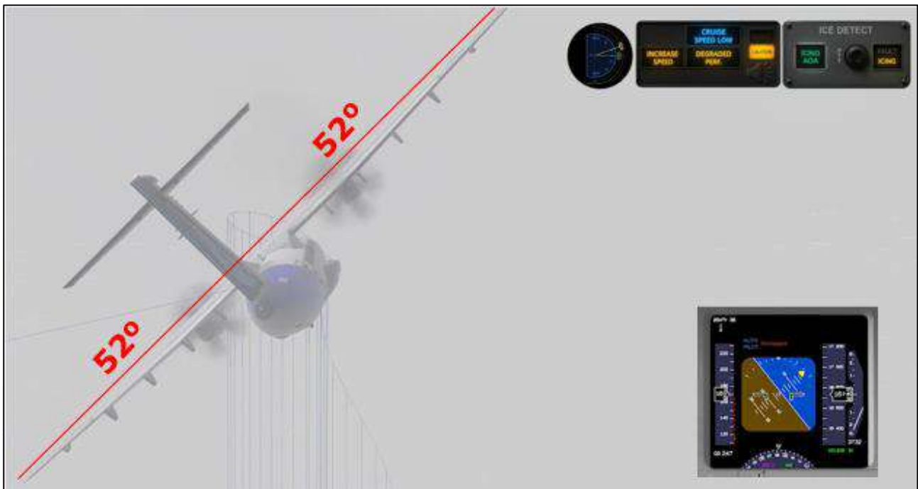
Figure 189 - Illustration demonstrating the 52° bank angle following the stall.
