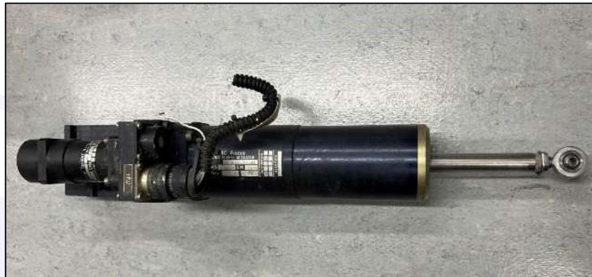
Figure 91 – Stick Pusher actuator prior to the start of examinations and tests, with the actuator rod in the extended position.
