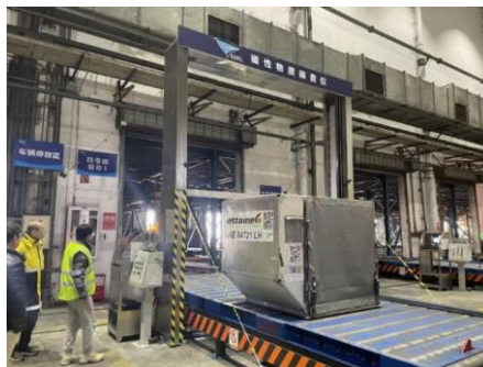
Figure 1. On-site implementation of rapid detection system for weak magnetic substances in large-scale cargo terminals
