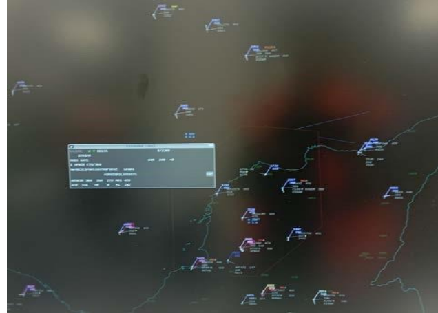
Figure 2. ADS-B/SSR Combined View
