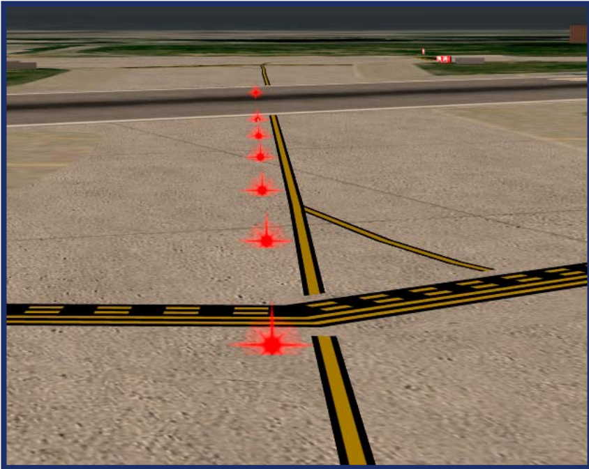
Runway Entrance Lights (RELs)
