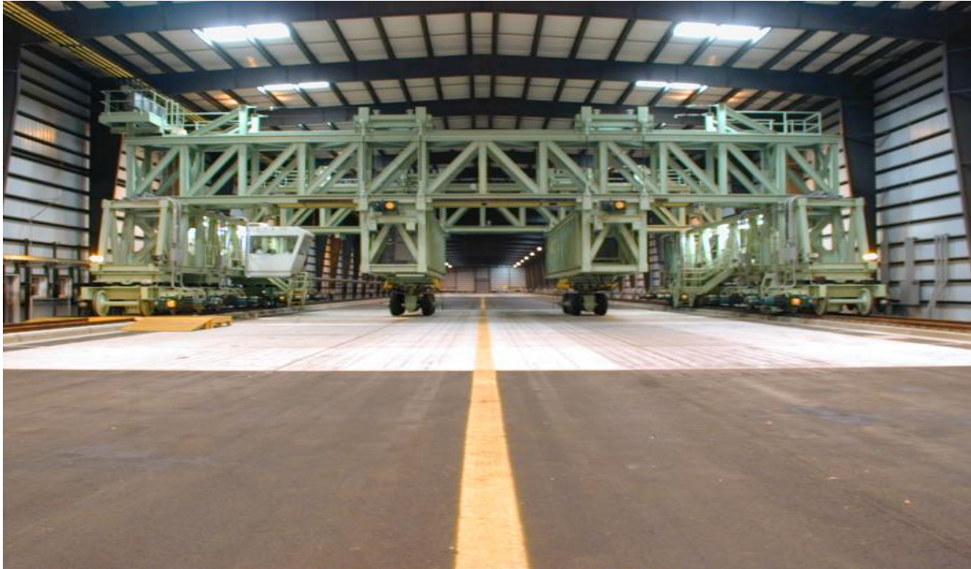
Instrumented Test Track at the NAPTF, FAA Technical Center
