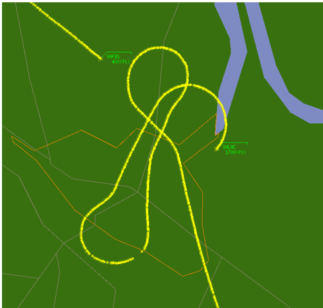
Figure 1. Two ADS-B aircraft 60 NM from the ADS-B ground station
