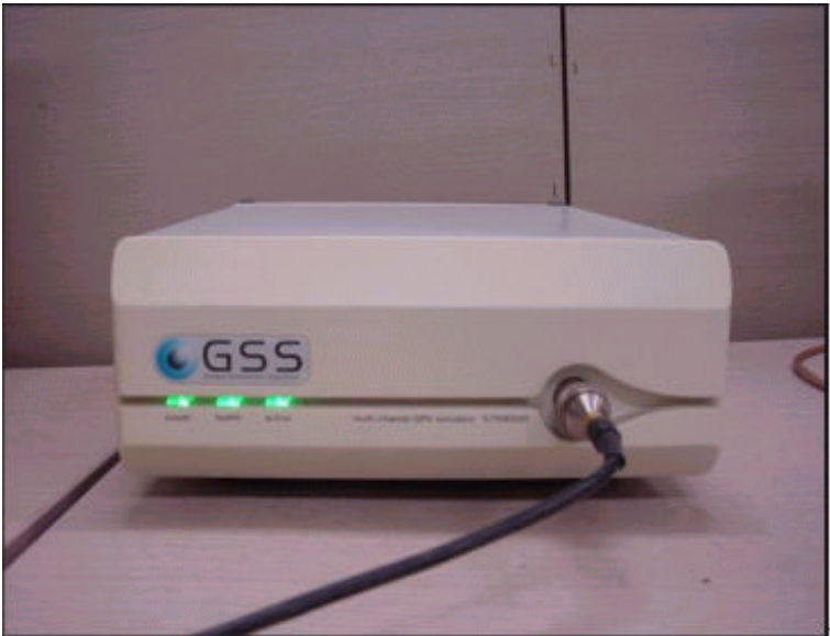
Figure 14. GNSS simulator: RF signal part
