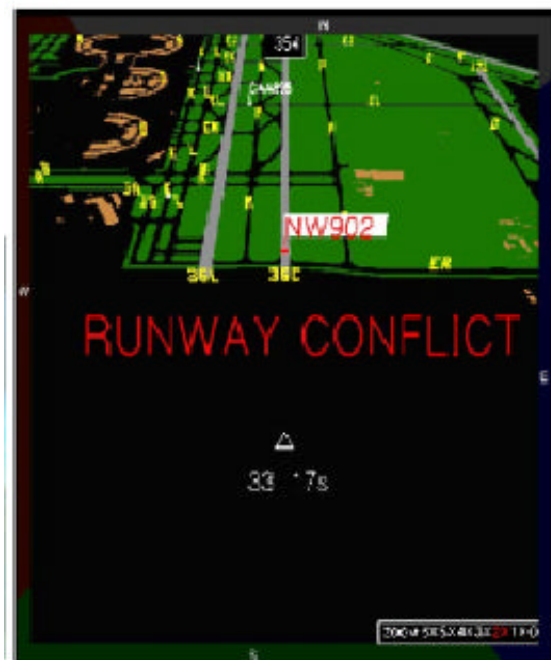
Figure 2. Cockpit arrival moving map display
