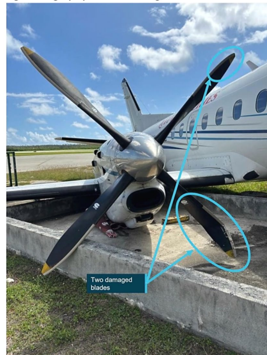
Figure 8: Right propeller blade damage
