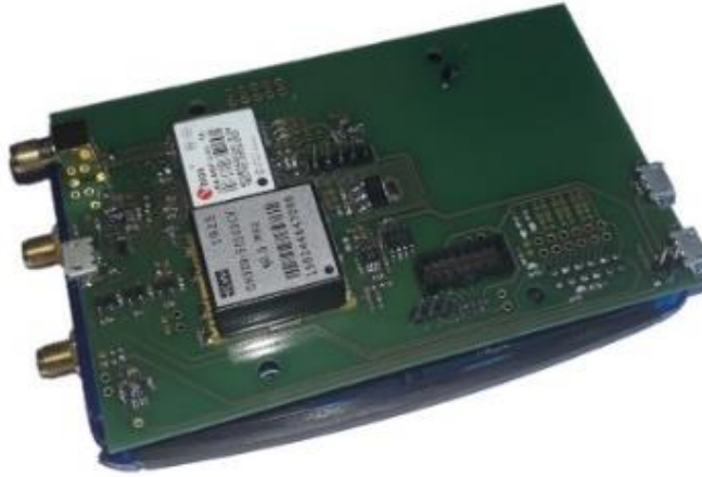
Figure 7. Adalm-Pluto SDR with added time synchronization board
