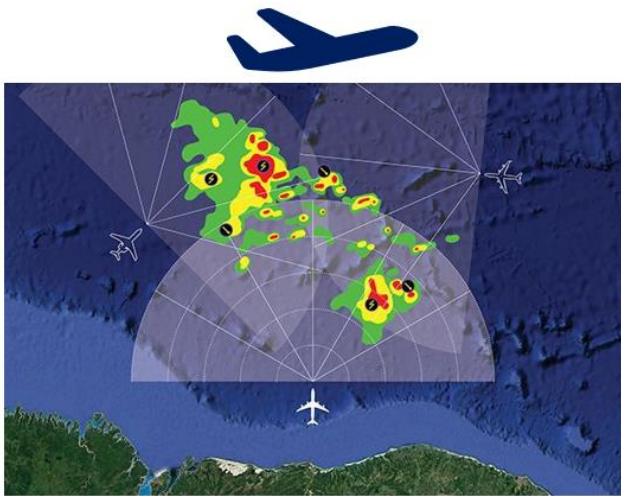
Figure 6. Composite Weather View Enabled by Connected Radar
