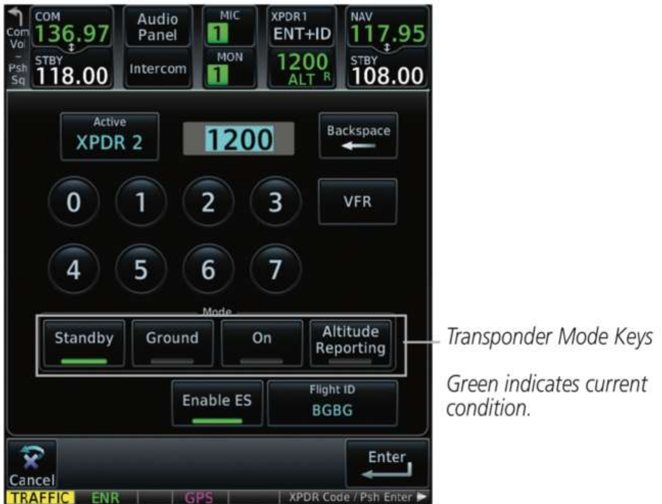
FIG 1: Example of a Sophisticated GA Panel – includes ability to transmit ADS-B with MODE S turned off.
