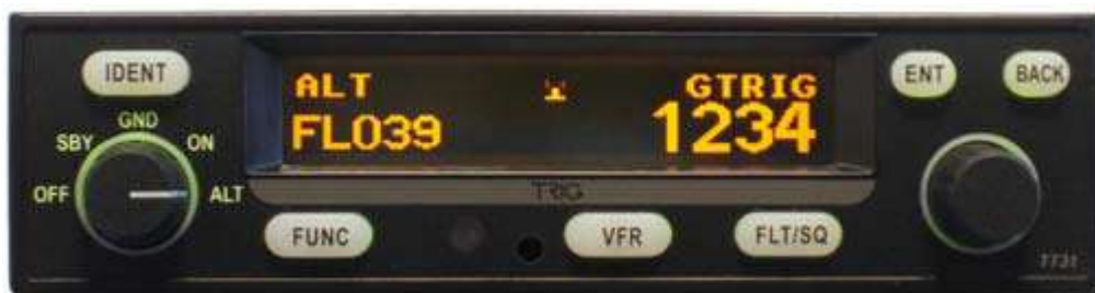
FIG 2: Example of a less sophisticated and more common GA Panel – ADS-B and MODE S in one transponder.
