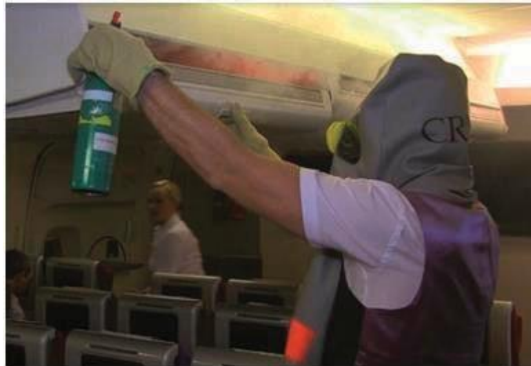
Figure 18 – Discharging a fire extinguisher into an overhead locker
