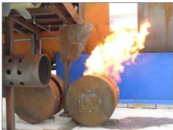
Landing gear fire
