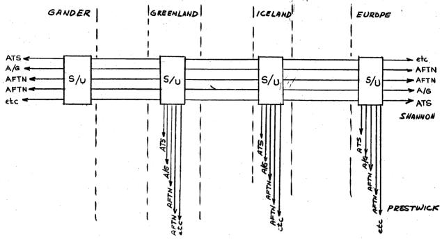
Although 5 "tails" have been shown at each location, any number may be connected, and this number would be one of the factors determining the capacity of the storage unit. With such an arrangement any tail would obtain the most rapid connexion with any other tail using any of the three sectors of the four channels which happened to be available.
