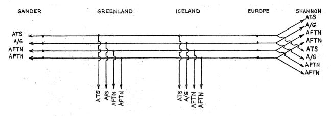
The disadvantages are apparent; there is no interconnexion between authorities, and on any circuit operation over the whole length may be interminably delayed by an operation over part of its length. It should further be noted that the number of authorities is limited to four.
