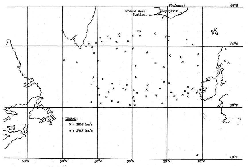
Aircraft positions on occasions when contact was only possible by ground wave
