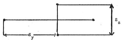
For such a pattern future improvements in altimetry will then improve lateral safety (although improvements in lateral accuracy will still decrease vertical safety). The alternative procedure would be to shift all alternate rows (tracks at same altitude) north (or south) by  $\frac{1}{2}$   $S_y$ . The symmetric basic pattern will then be:
