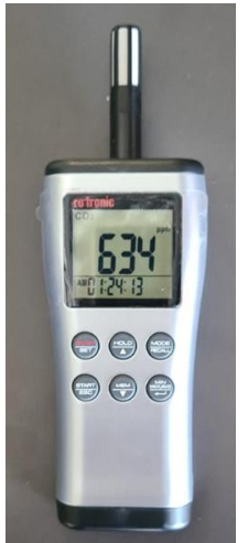
CO2 measurement device with alert level
