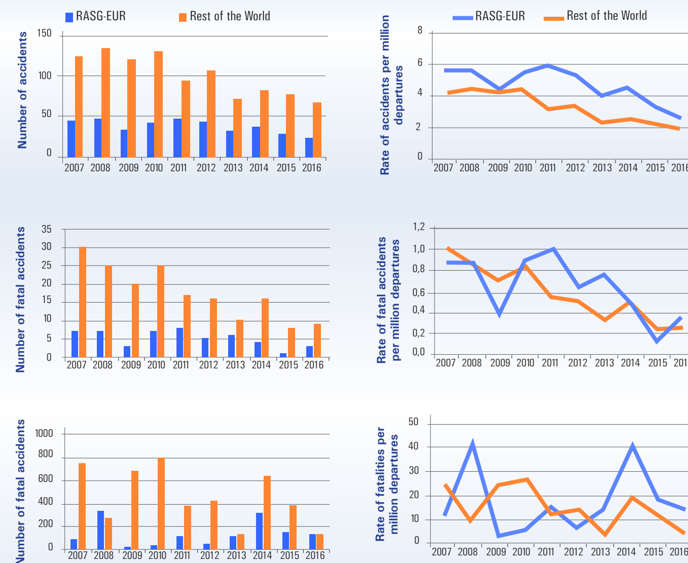
Figure 3: Number and rate of accidents, fatal accidents and fatalities in the ICAO EUR region, compared with the rest of the world, scheduled commercial air transport aeroplanes above 5,700 kg (source: EASA)
