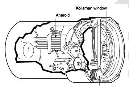
Barometric scale adjustment knob
