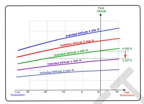
Note: The diagram shows the relation between the indicated altitude and the temperature variation from ISA.
