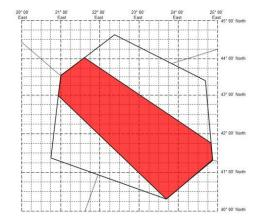
YUDD SIGMET 2 VALID 101200/101600 YUSO— YUDD SHANLON FIR SEV TURB FCST NE OF LINE N4300 E02057 — N4020 E02340 AND SW OF LINE N4402 E02142 — N4145 E02450 FL250/370 MOV NE 20KT WKN=
