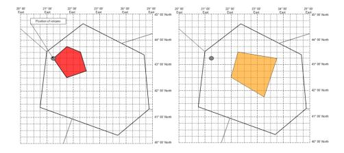
YUDD SIGMET 2 VALID 101200/101800 YUSO— YUDD SHANLON FIR/UIR VA ERUPTION MT ASHVAL PSN N4315 E02115 VA CLD OBS AT 1200Z WI N4315 E02115 — N4345 E02145 N4330 E02215 — N4245 E02230 — N4230 E02145 - N4315 E02115 FL250/370 NC FCST AT 1800Z WI N4330 E02215 — N4315 E02345 — N4145 E02315 — N4230 E02200 - N4330 E02215=
