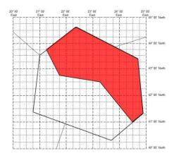
YUDD SIGMET 2 VALID 101200/101600 YUSO— YUDD SHANLON FIR SEV TURB FCST NE OF LINE N4345 E02115 — N4245 E02145 - N4230 E2315 — N4100 E2430 FL250/370 WKN FCST AT 1600Z NE OF LINE N4411 E02145 — N4255 E02228 - N4228 E2400 — N4130 E2450=
