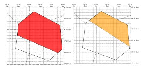
YUDD SIGMET 2 VALID 101200/101600 YUSO— YUDD SHANLON FIR SEV TURB FCST NE OF LINE N4230 E02052 – N4100 E02430 FL250/370 WKN FCST AT 1600Z NE OF LINE N4346 E02122 – N4130 E02452=
