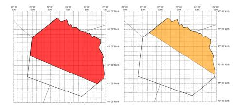
YUDD SIGMET 2 VALID 101200/101600 YUSO— YUDD SHANLON FIR SEV TURB FCST NE OF LINE N4230 E02052 – N4100 E02430 FL250/370 WKN FCST AT 1600Z NE OF LINE N4346 E02122 – N4130 E02457=
