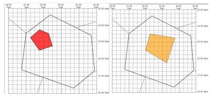
YUDD SIGMET 2 VALID 101200/101600 YUSO— YUDD SHANLON FIR/UIR TEST SEV TURB FCST WI N4230 E02145 – N4315 E02115 – N4345 E02145 – N4330 E02215 – N4245 E02230 - N4230 E02145 FL250/370 INTSF FCST AT 1600Z WI N4145 E02315 – N4230 E02200 – N4330 E02215 – N4315 E02345 - N4145 E02315=
