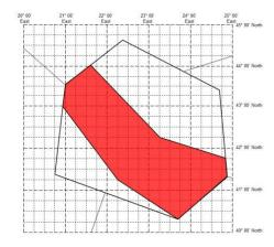
YUDD SIGMET 2 VALID 101200/101600 YUSO— YUDD SHANLON FIR SEV TURB FCST NE OF LINE N4300 E02057 – N4115 E02215 – N4020 E02340 AND SW OF LINE N4402 E02142 – N4215 E02315 - N4145 E02450 FL250/370 MOV NE 20KT WKN=
